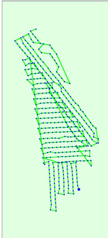
Figure 2: Top view of the initial image position. The green line follows the position of the images in time starting from the large blue dot.
