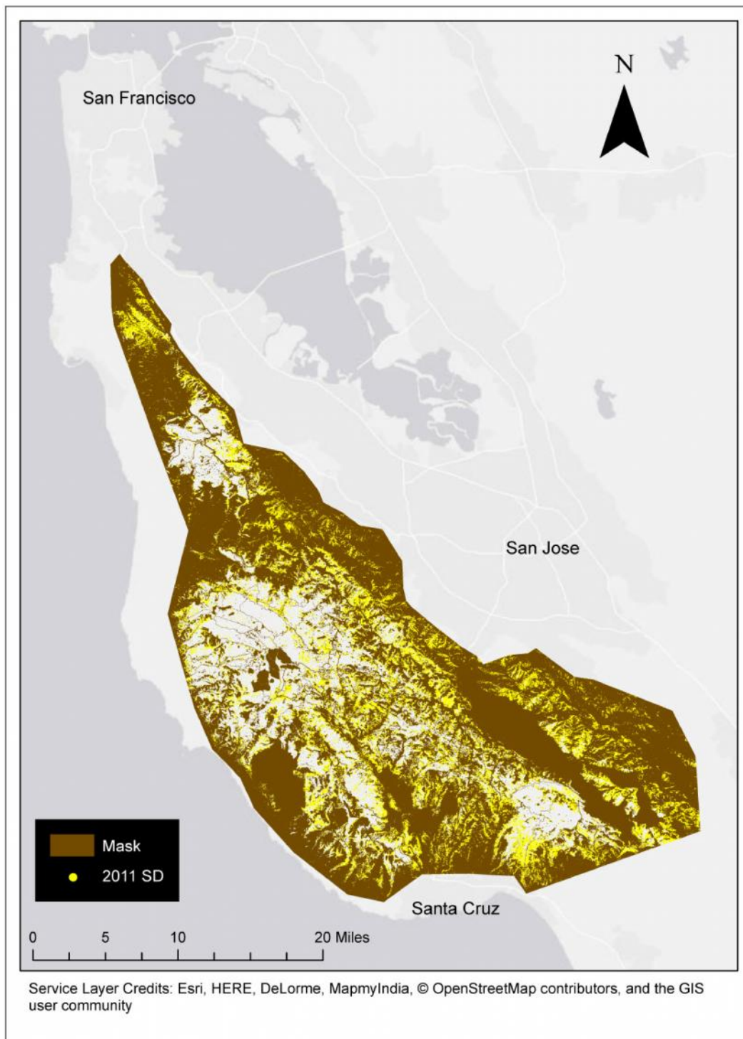
Figure C18 The extent of serious tree death in 2011. Each pixel classified as SD is displayed as a single yellow point. Non-forested areas, masked out, are shown in brown.
