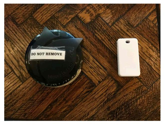
Figure 7 BlueCats BC 313 beacon (76mm x 27.80mm) on left, and coin beacon (52mm x 27mm x 7mm) on right used in project
