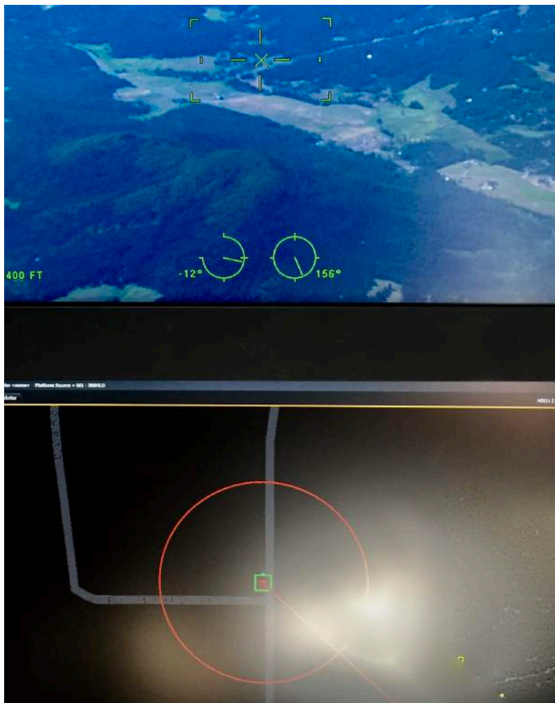
Figure 12 Road Data verify correct location. The green X above is paired with the center of the red circle, giving the user situational awareness that they are looking at the correct target.
