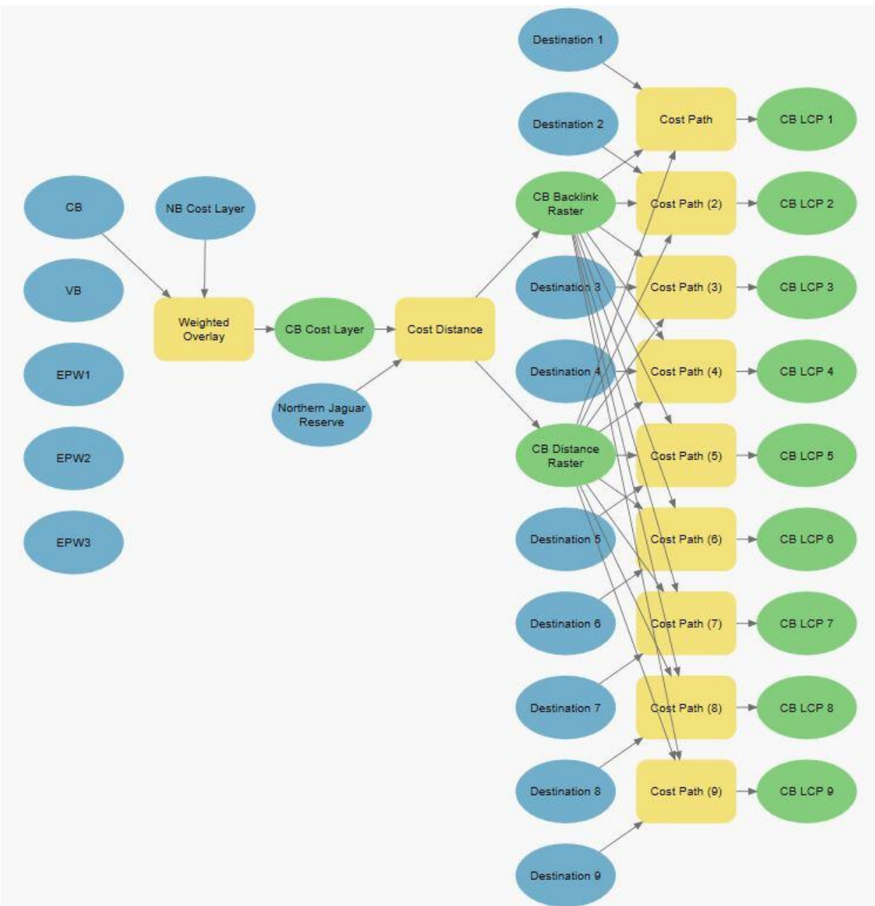
Figure 16. Model for the creation of the LCPs. This iteration shows the CB scenario being run
