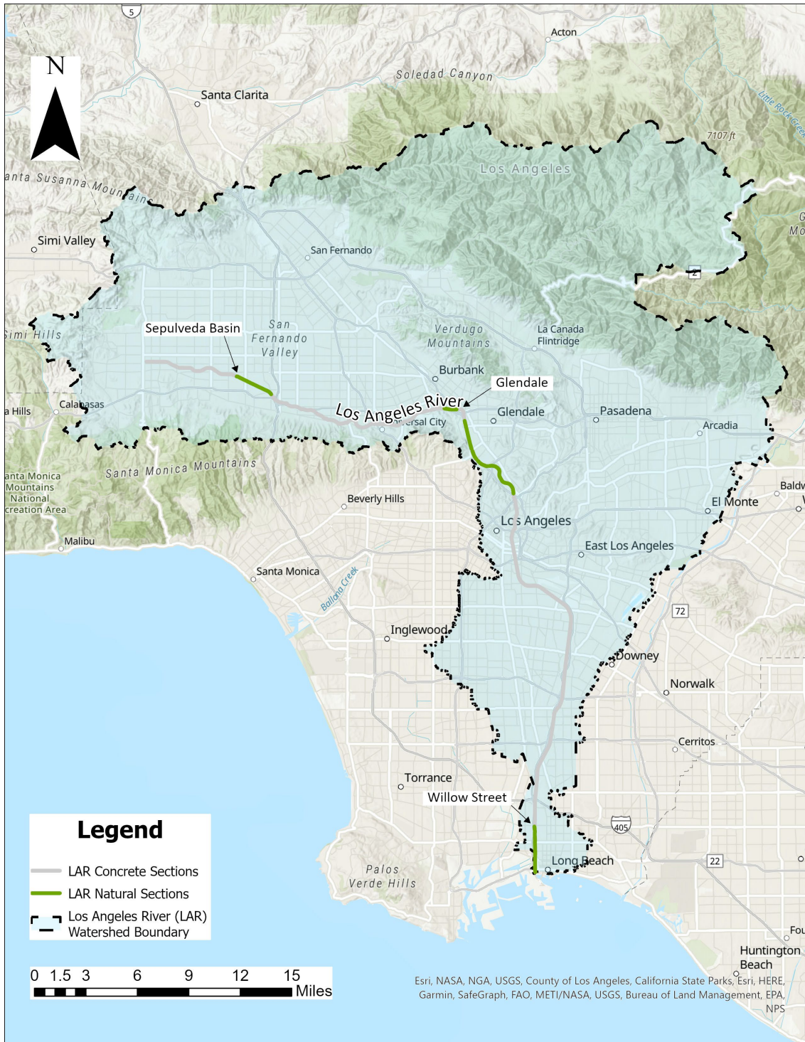
Figure 2. Concrete and natural reaches of LAR
