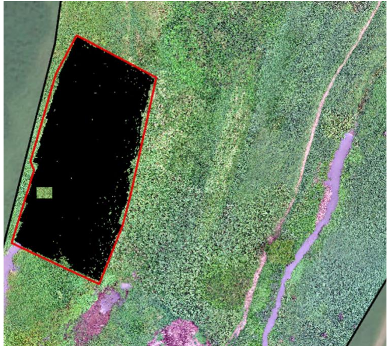
Figure 11: A blackout spot, or area with “No Data” created from Pix4D
