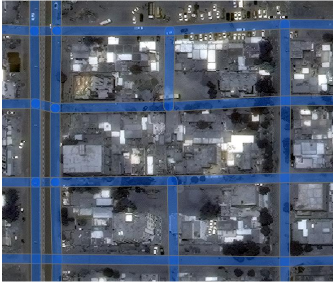
Figure 7: Road labels created from three-meter buffers. The three-meter buffer appears to fit the roads in Khartoum well - any wider and the label would likely start catching too many non-road pixels and cause false positives.
