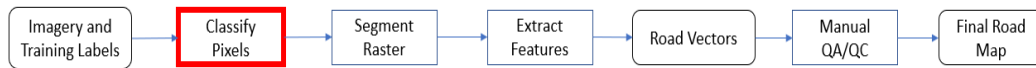
Figure 1: Road extraction workflow. This project focuses on optimizing the ‘Classify Pixels’ step.
