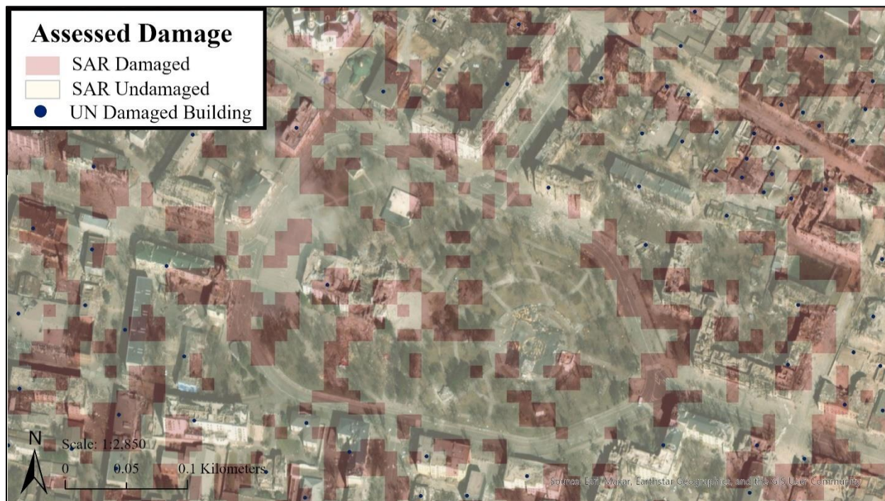
Figure 39. SAR damage polygons and UNOSAT damage points over Mariupol drama theatre
