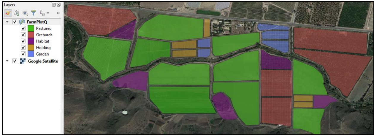
Figure 13. The spatial attributes of the FarmPlot table created as a polygon shapefile in QGIS.
