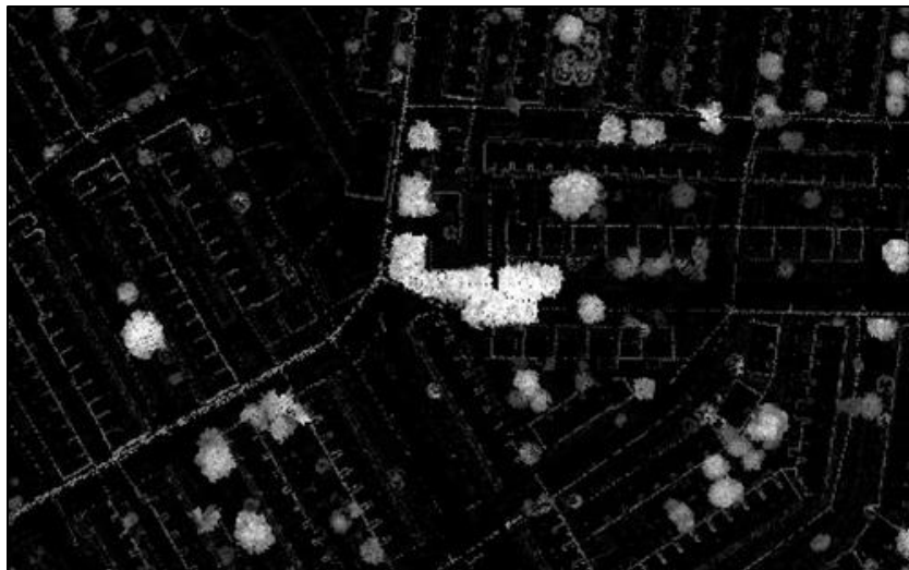
Figure 5. Standard deviation of LiDAR point cloud elevation. Image from O’Neil-Dunne et al. (2013)
