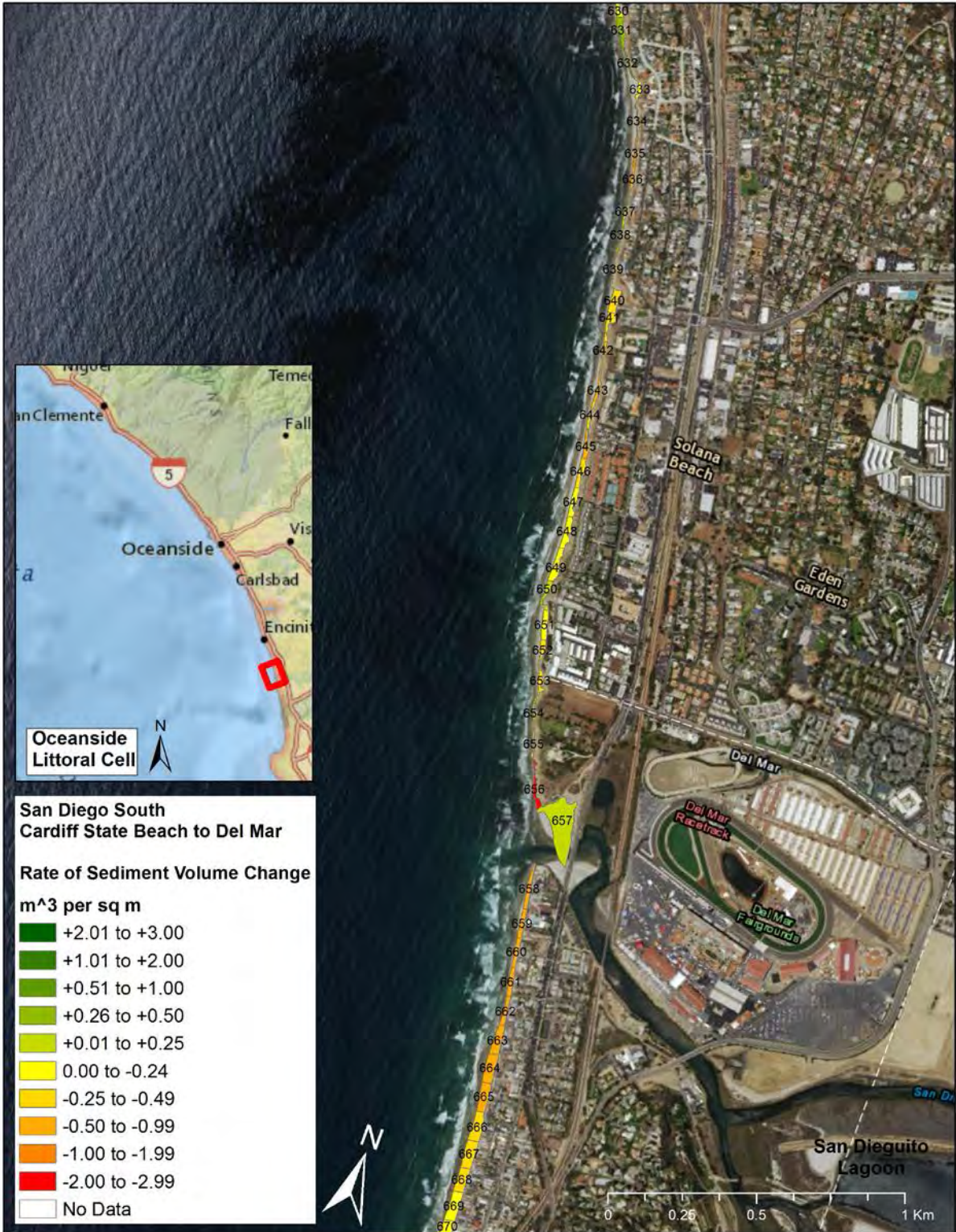
Figure 76 Cardiff State Beach to Del Mar - Map of rate of sediment volume change by shore segments during the 06-07 El Niño
