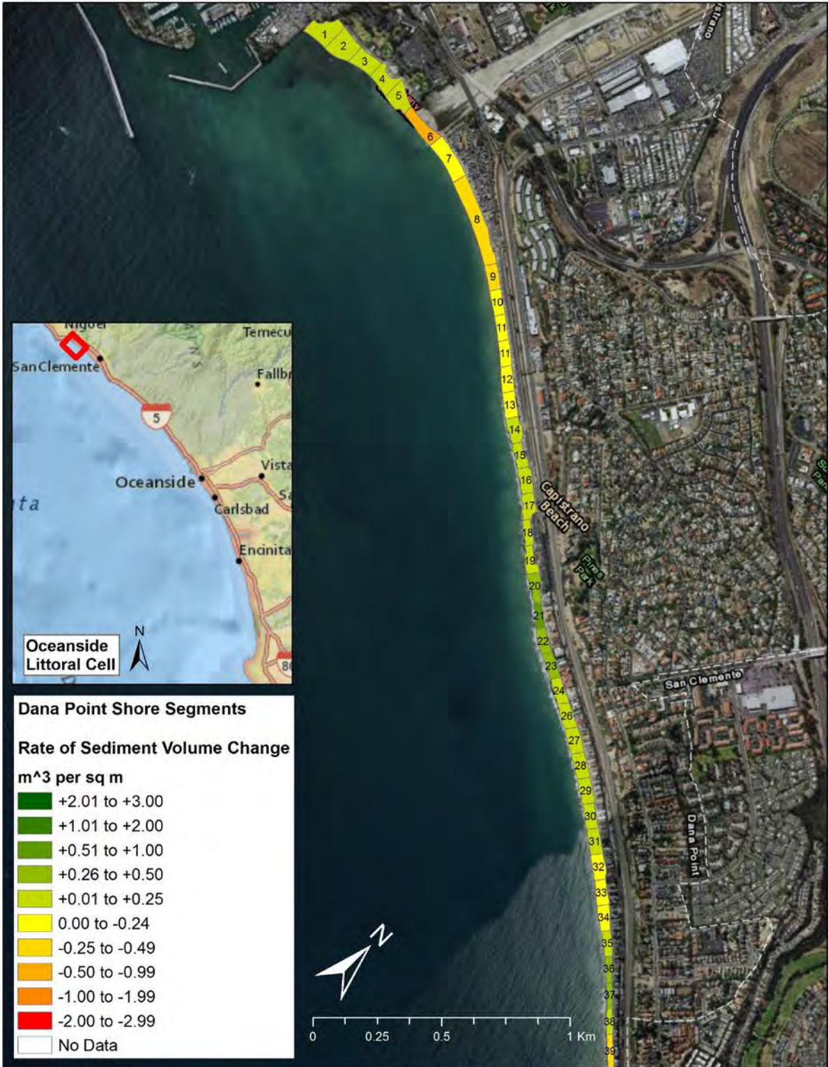
Figure 26 Dana Point - Map of rate of sediment volume change by shore segments during the 06-07 El Niño
