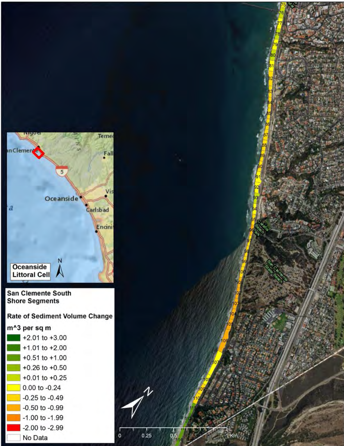
Figure 32 San Clemente (South) - Map of rate of sediment volume change by shore segments during the 06-07 El Niño
