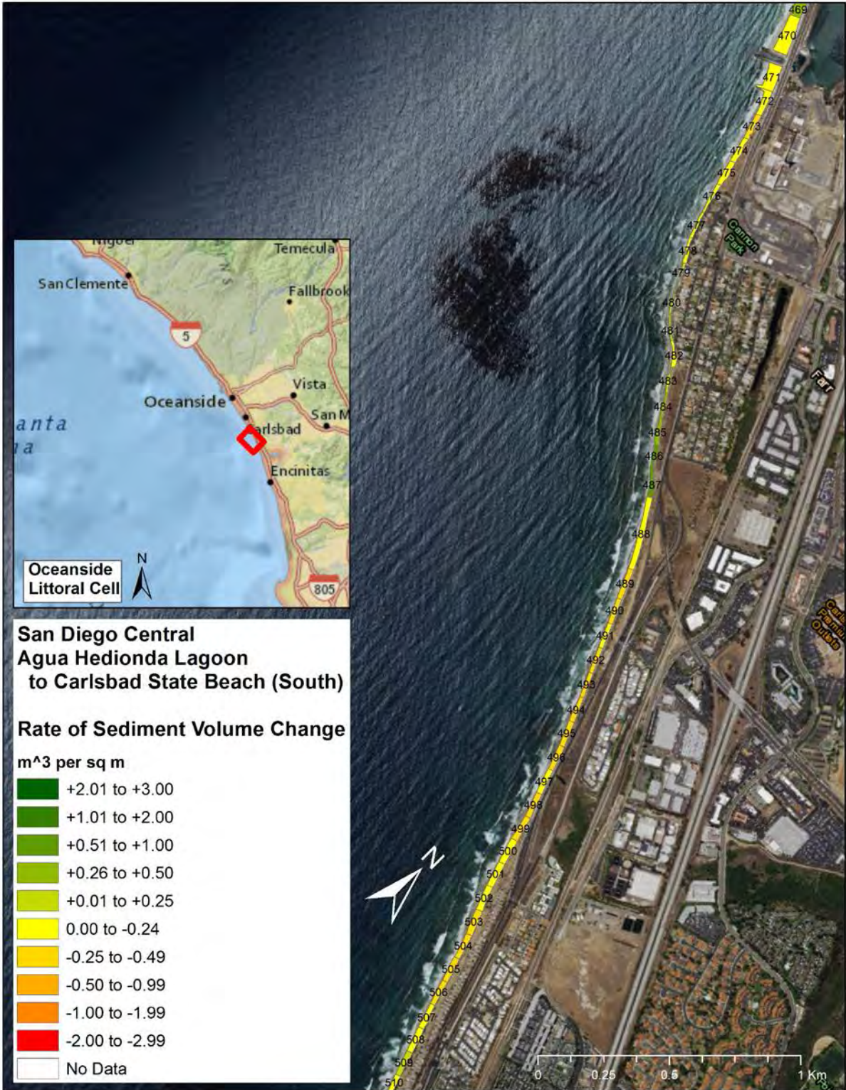
Figure 64 Carlsbad State Beach (Agua Hedionda Lagoon) to Carlsbad State Beach (South) - Map of rate of sediment volume change by shore segments during the 06-07 El Niño
