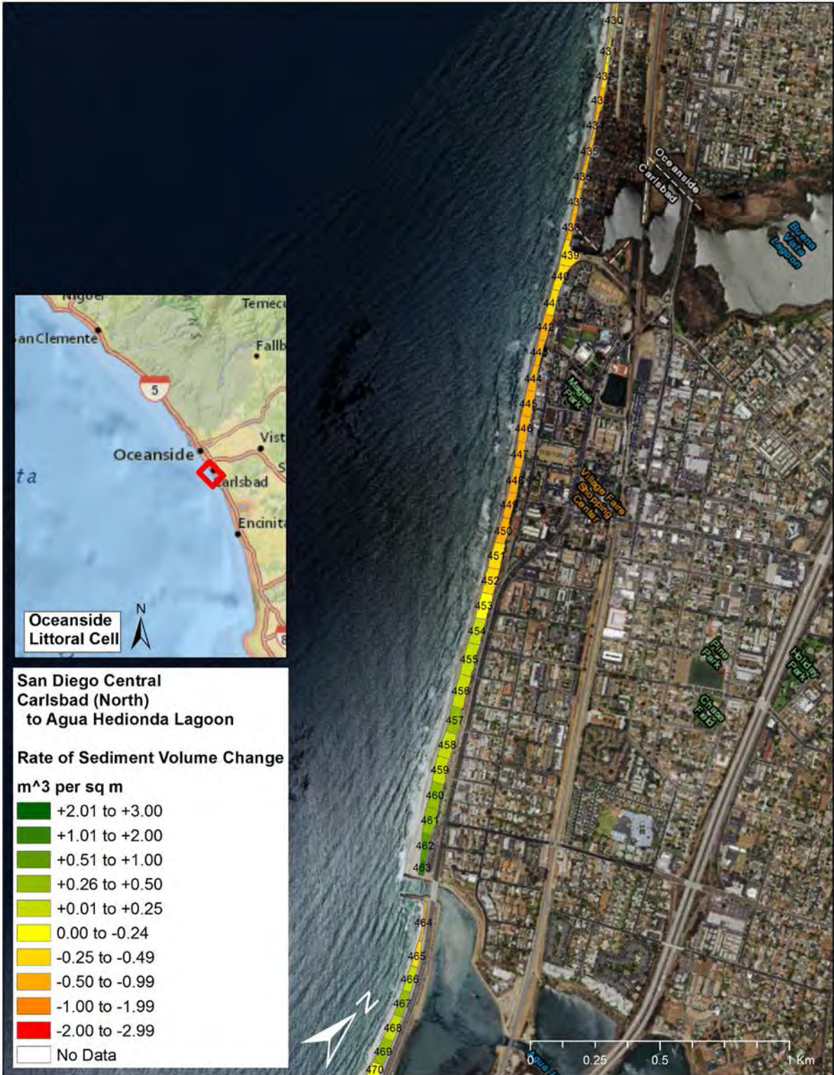
Figure 61 Carlsbad North to Carlsbad State Beach (Agua Hedionda Lagoon) - Map of rate of sediment volume change by shore segments during the 06-07 El Niño
