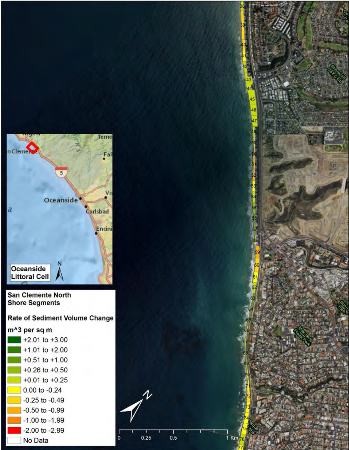
Figure 29 San Clemente (North) - Map of rate of sediment volume change by shore segments during the 06-07 El Niño
