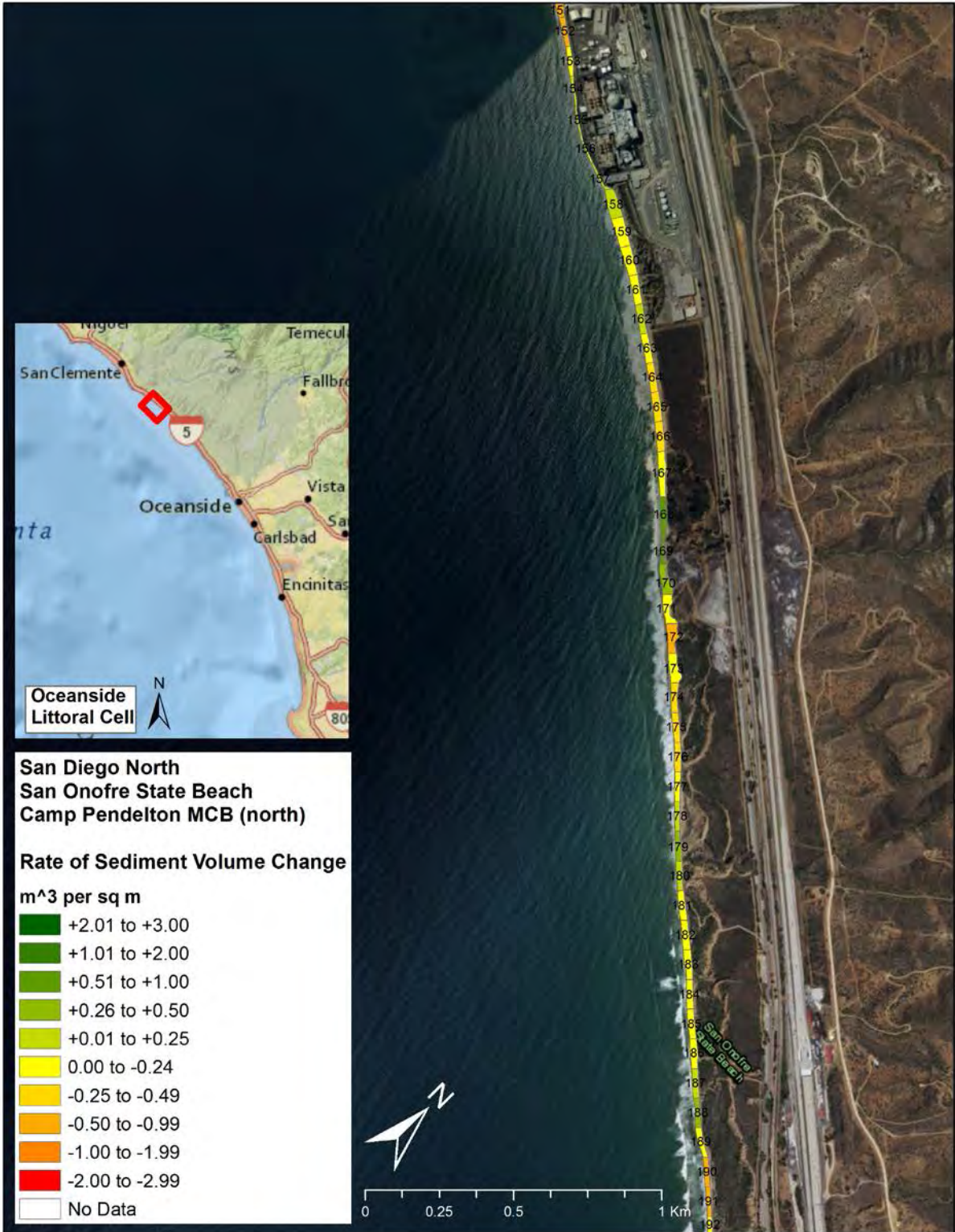
Figure 38 San Onofre State Beach to Camp Pendelton MCB (North) - Map of rate of sediment volume change by shore segments during the 06-07 El Niño
