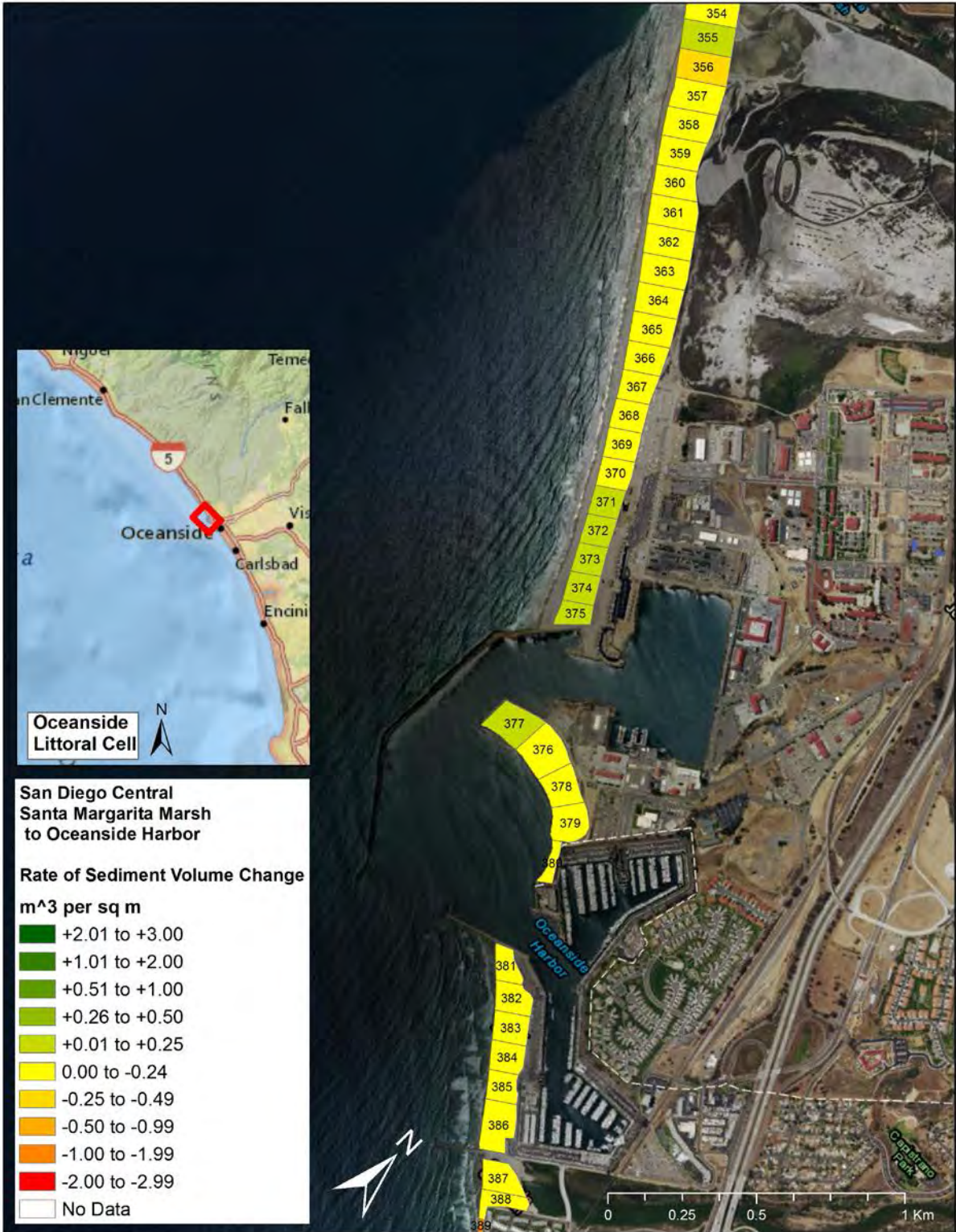
Figure 55 Santa Margarita Marsh to Oceanside Harbor - Map of rate of sediment volume change by shore segments during the 06-07 El Niño
