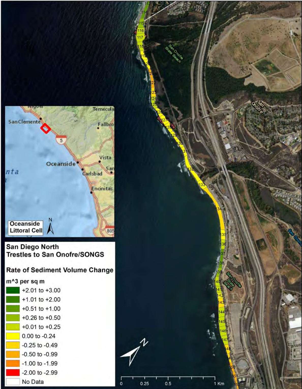
Figure 35 Trestles to San Onofre (SONGS) - Map of rate of sediment volume change by shore segments during the 06-07 El Niño
