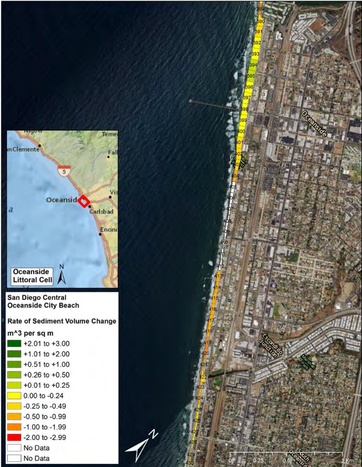
Figure 58 Oceanside City Beach - Map of rate of sediment volume change by shore segments during the 06-07 El Niño
