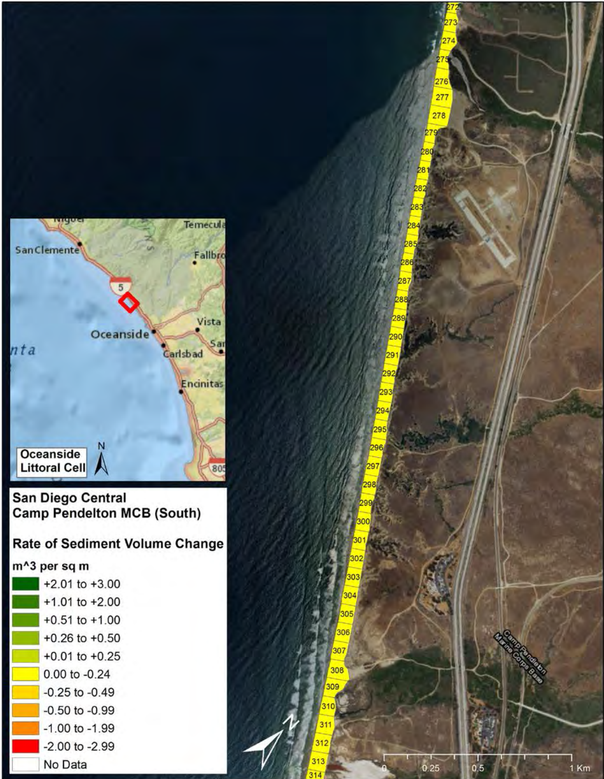
Figure 48 Camp Pendelton MCB (South) - Map of rate of sediment volume change by shore segments during the 06-07 El Niño
