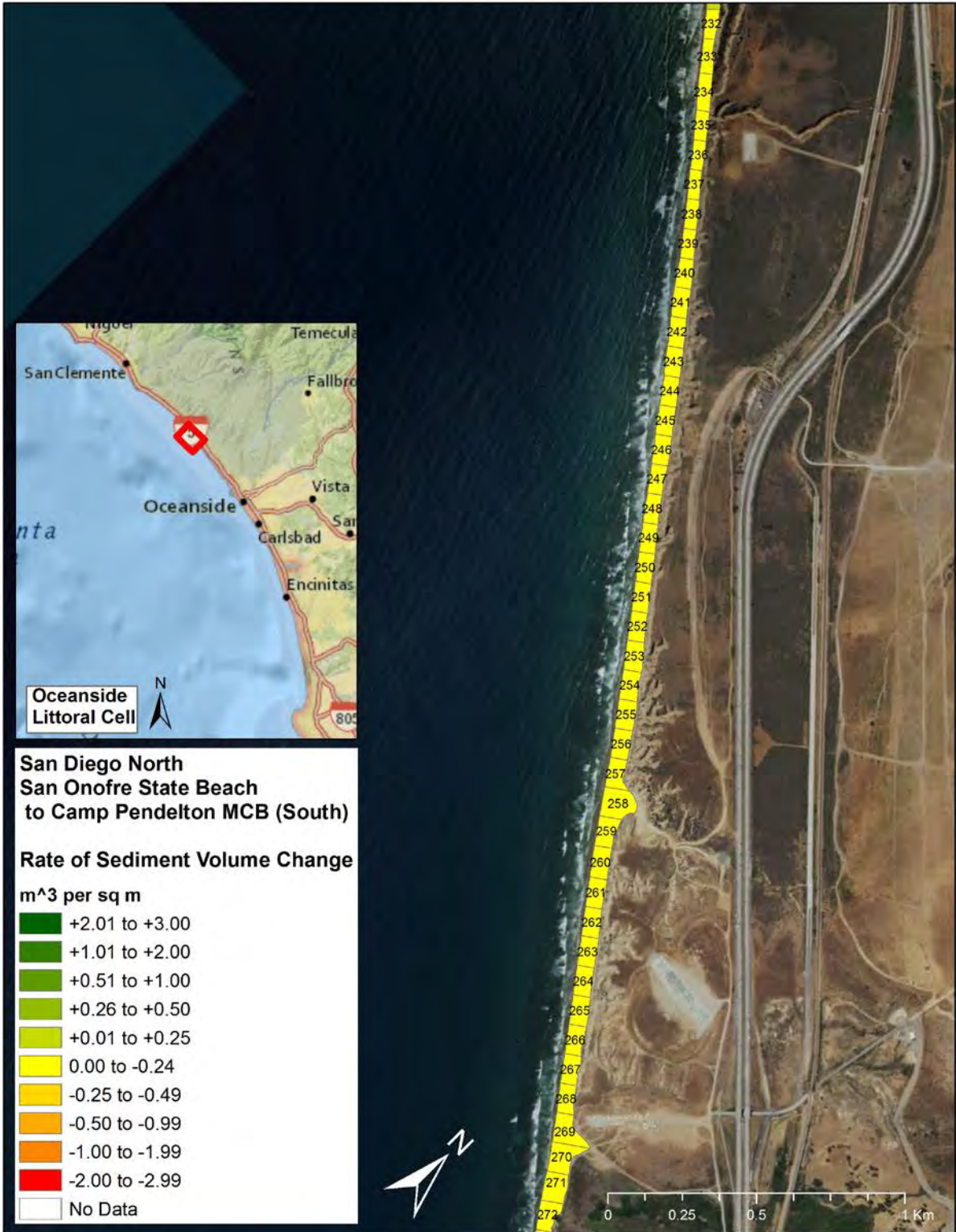
Figure 45 San Onofre State Beach/Camp Pendelton MCB (South) - Map of rate of sediment volume change by shore segments during the 06-07 El Niño
