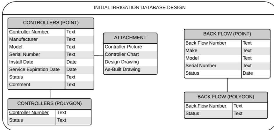
Figure 6 Irrigation Database Design
