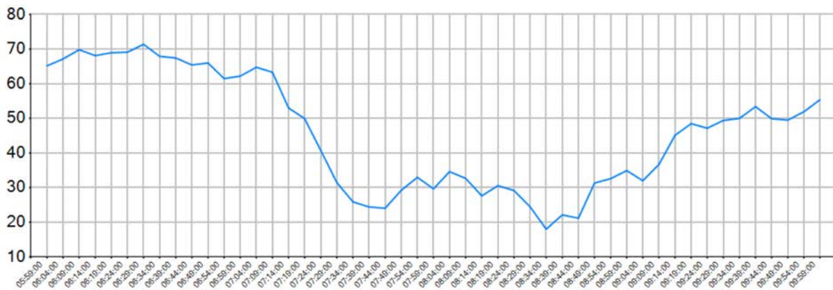
Figure 19: Typical Pattern for Freeways from 0600-1000. This graph is from I-10W at Washington Blvd. Free flow speed: 63 mph. MinuteAvgCF denotes average continuous flow (CF) for each minute.
