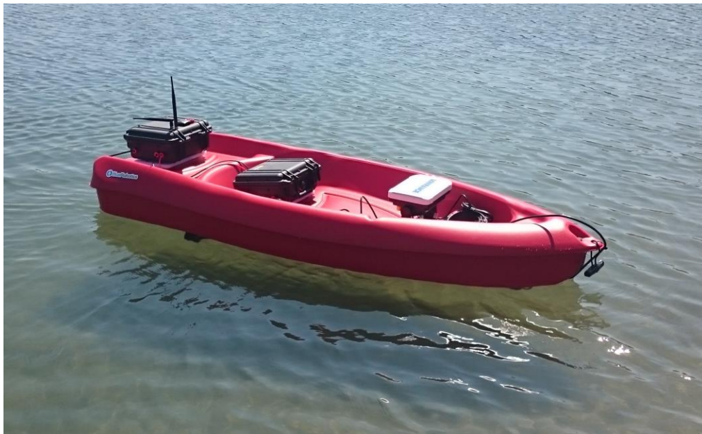
Figure 3.2 Completed USV with sonar, battery and navigation box.
