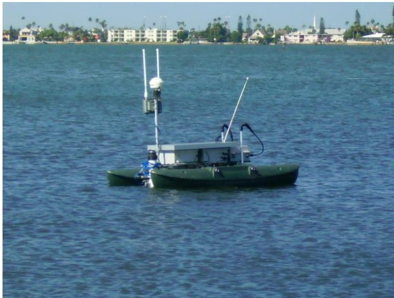
Figure 2.6 University of South Florida USV used for imaging eelgrass (Source: Dreger 2010 )
