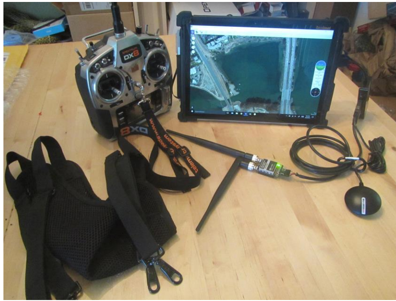
Figure 3.3 Image of Ground Control Station equipment: Chest Harness, Radio Control, Surface Pro 4, RFD 900+ and GPS receiver.
