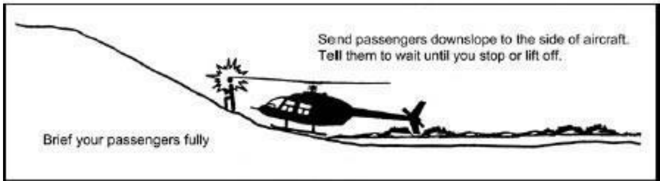
Figure 8 Hazards of Sloped HLZs to Personnel (Department of Transport, Canada 2006)
