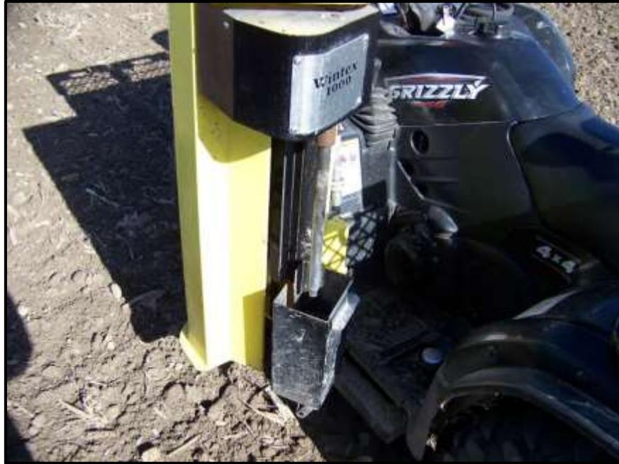
**Figure 15:** Automatic soil sampler mounted on ATV
