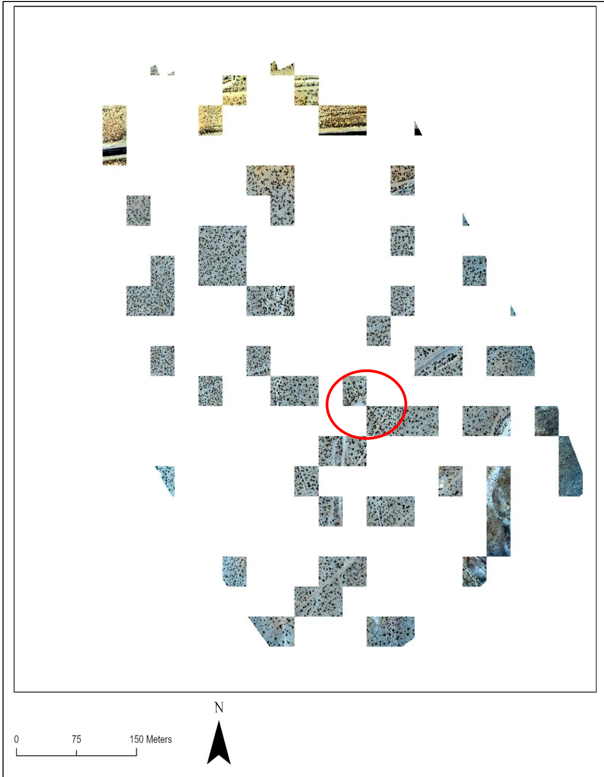
Figure 10 Randomized 30x30m rasters used for Test Run 4. Circled area shown in closer detail in Figure 12.
