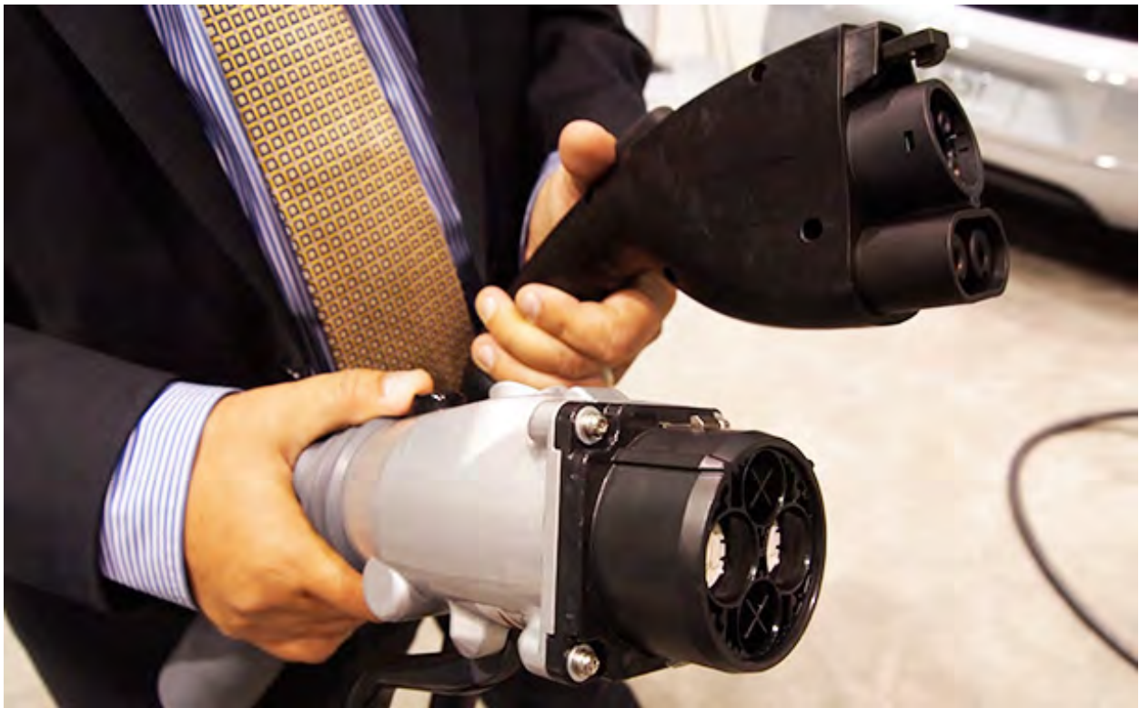
Figure 4 Two Common DC Fast Charging Plug. Source: Birdman 2014
