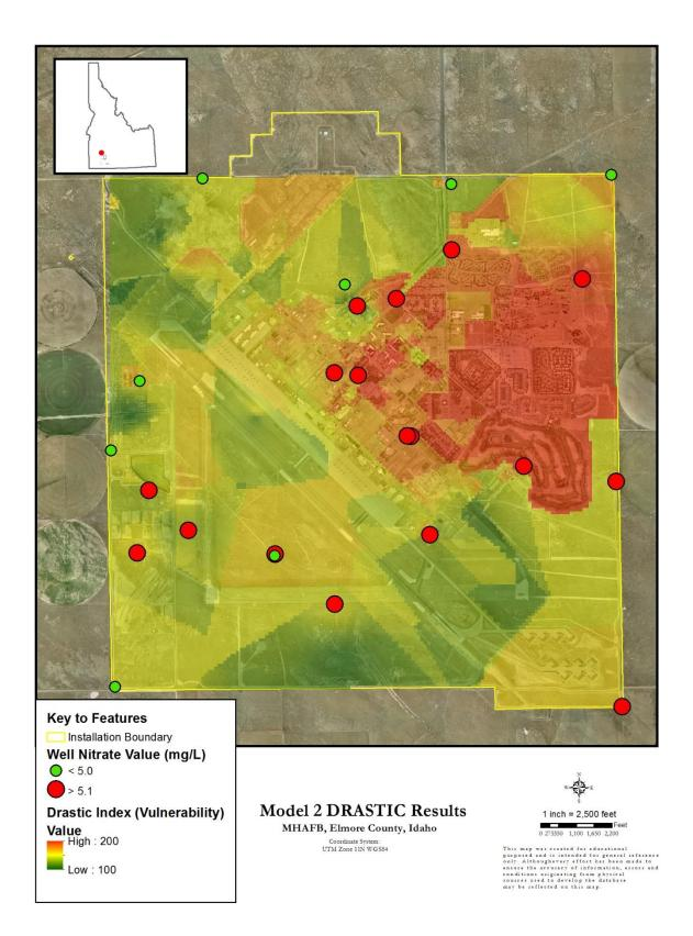
Figure 14. Model 2 – DRASTIC Index of vulnerability for Mountain Home AFB, using site-specific data and overlaid with average nitrate sampling results per well.
