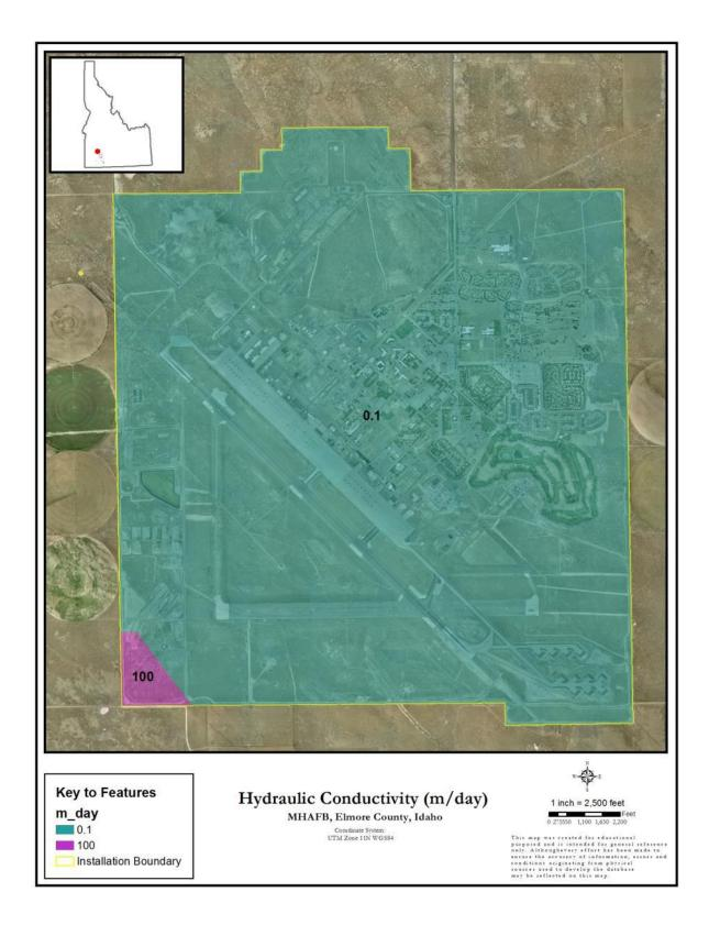
Figure A 4. DRASTIC Parameter Hydraulic Conductivity, using generic, available data.
