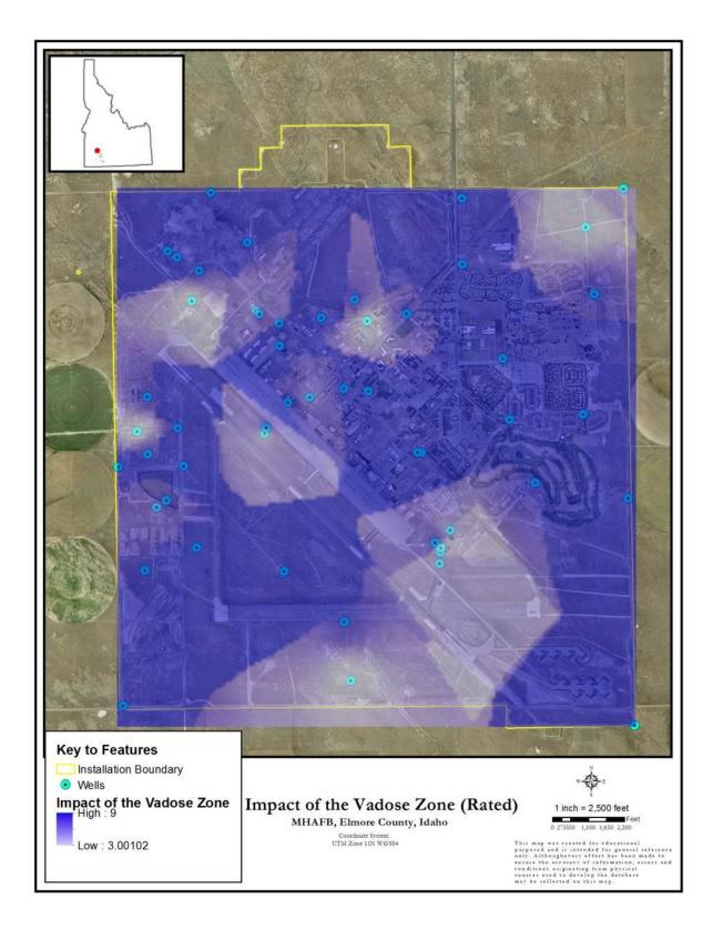
Figure 12. Impact of the Rated Vadose Zone, ranging from 9 to 3. Data obtained from well driller's logs. Wells are depicted in blue.
