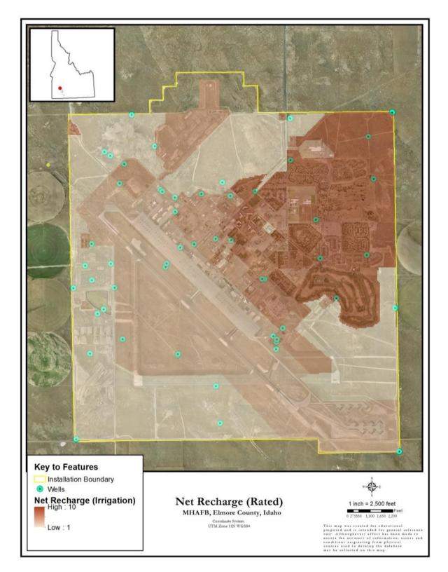
Figure 11. Site-specific land cover type to obtain Rated Net Recharge, ranging from Urban/Developed Land (darker red) to barren, rangeland (white). Wells are depicted in blue. if any, involved with these land uses. The area with the greatest amount of irrigation use is the golf course, which uses an average of 1 to 2 million gallons of water per day during the growing season (rating score 10).
