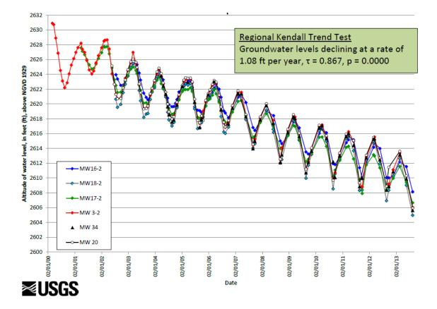
Figure 2. Altitude of water level, in feet (ft), above NGVD 1929 indicating groundwater levels declining at a rate of 1.08 ft per year *Source:* Williams (2014)
