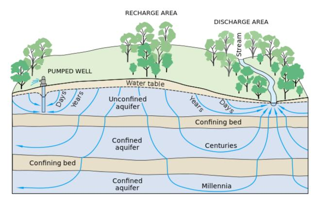
Figure 3. Water infiltrating the subsurface flows through the groundwater system and eventually discharges in streams, lakes, oceans, or is pumped from a well. The residence time in the subsurface can vary from days to thousands of years (Winter et al. 1998).
