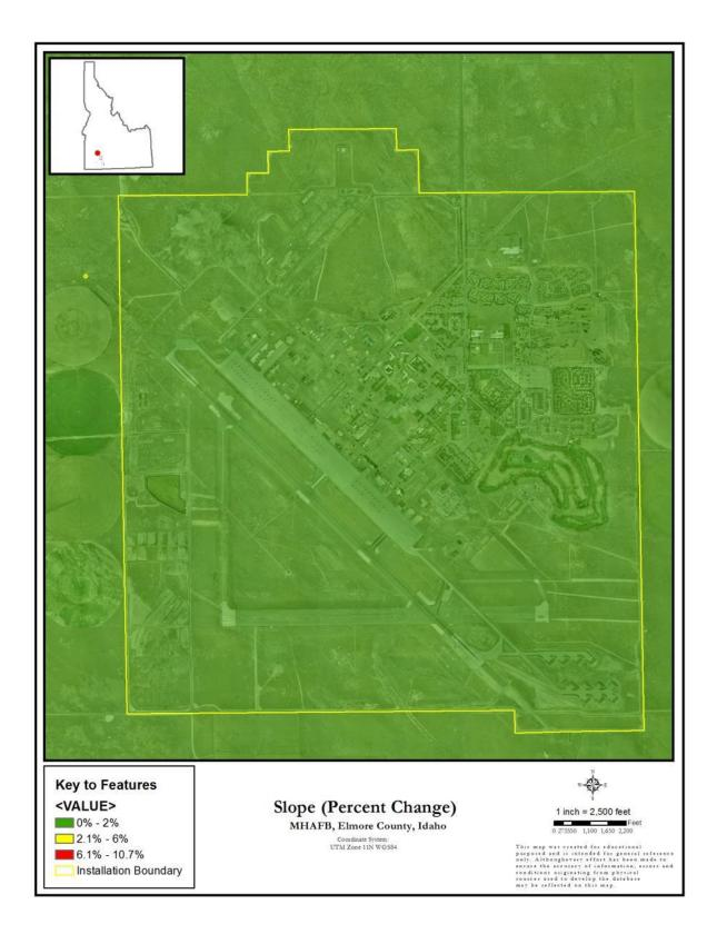
Figure A 2. DRASTIC Parameter Topography (Slope), using contour elevation data.
