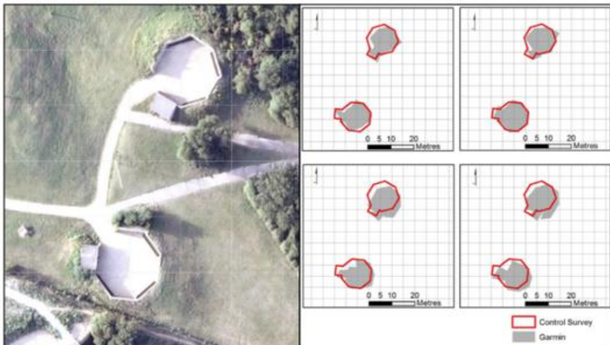
Figure 5: Accuracy comparison of survey grade and recreational GNSS devices (Haklay 2010)
