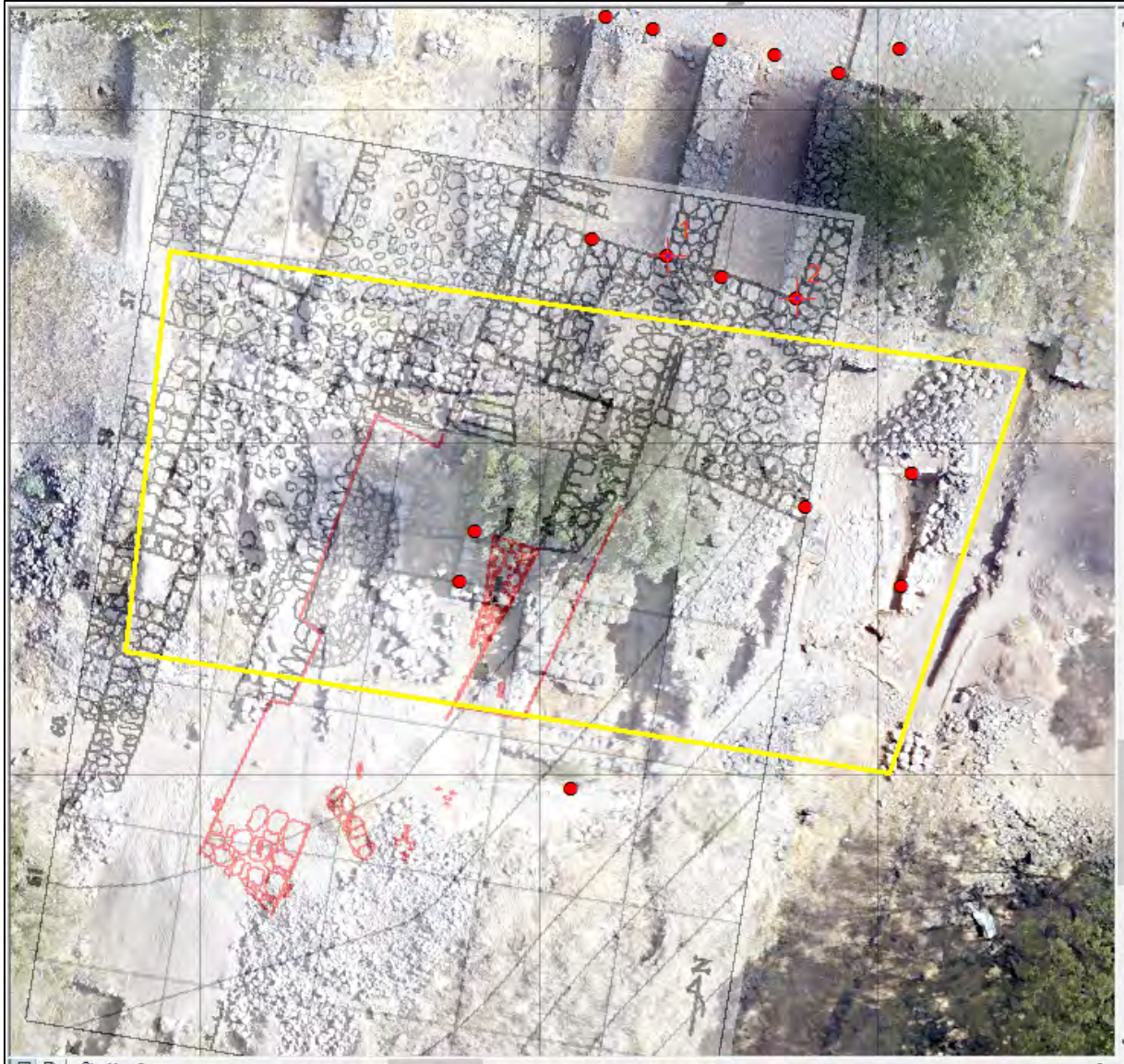
Figure 21. CAD drawing overlay in ArcMap at 40% transparency - Area A (South). Note the accuracy in the alignment of the corners of the granary bins at the top of the map
