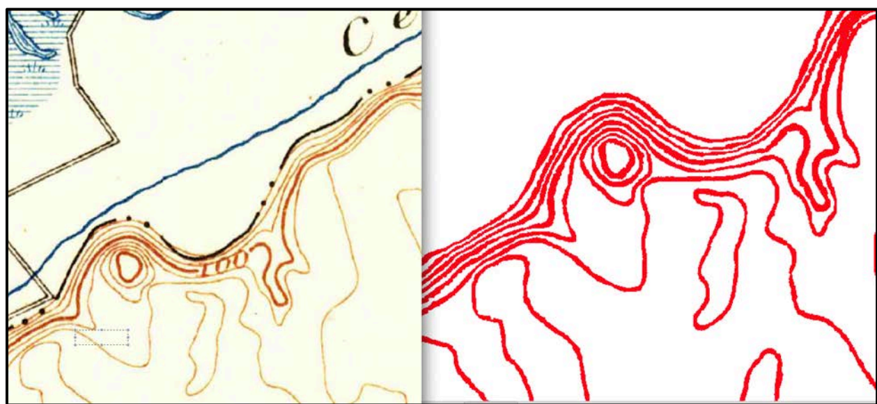
Figure 12. An example of manually cleaning contour lines in GIMP.
