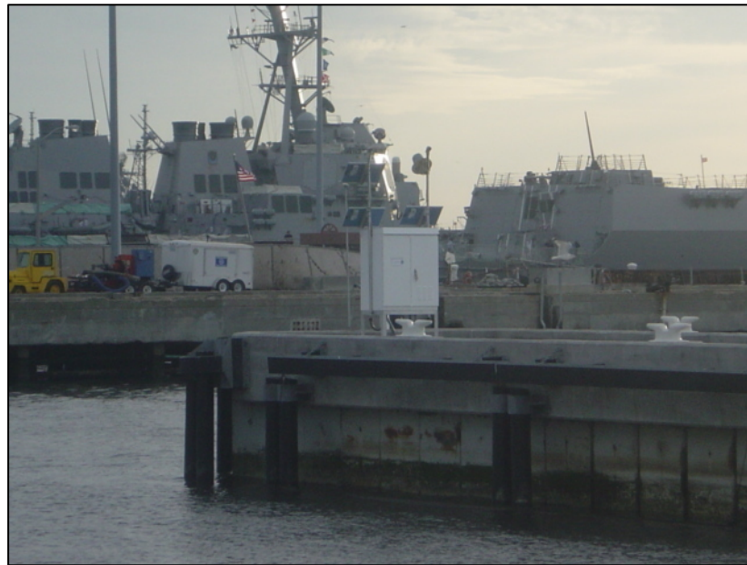
Figure 8 NOAA Primary Tide Gauge Installed at Sewells Point, VA (Source: National Oceanic and Atmospheric Administration 2015c)
