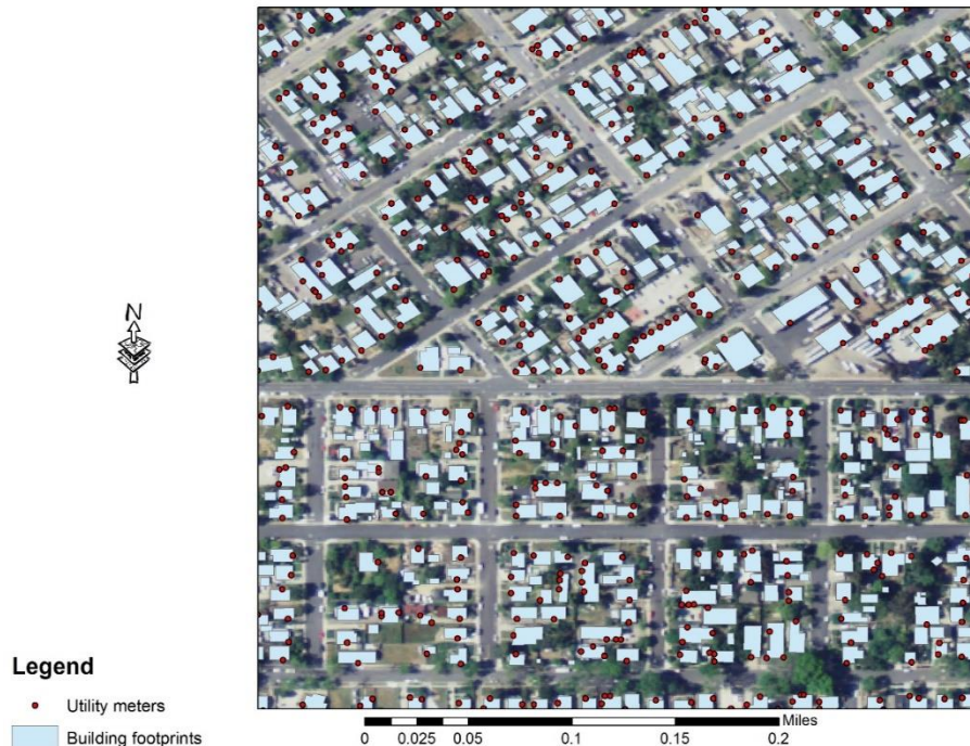
Figure 9: Map showing utility meters snapped to the nearest edge of the building footprints in a part of the City of San Luis Obispo
