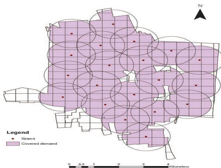
Figure 4: Murray and Tong's (2007) siren network coverage of demand regions in Dublin, OH
