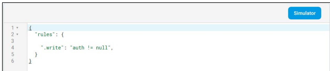
Figure 4.10 Realtime Database rules for authenticated user write access
