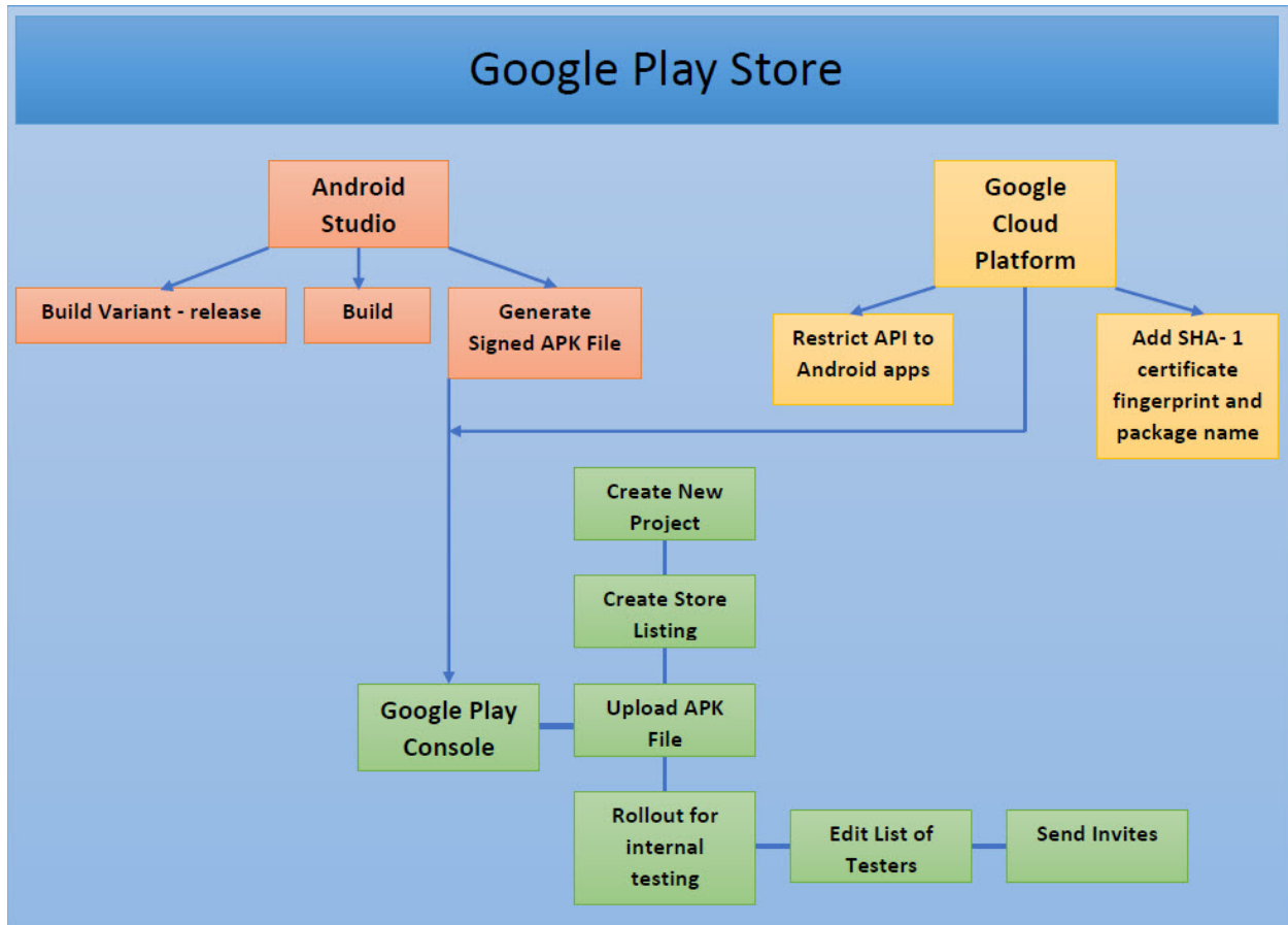
Figure 5.9 Process to deploy application for internal testing
