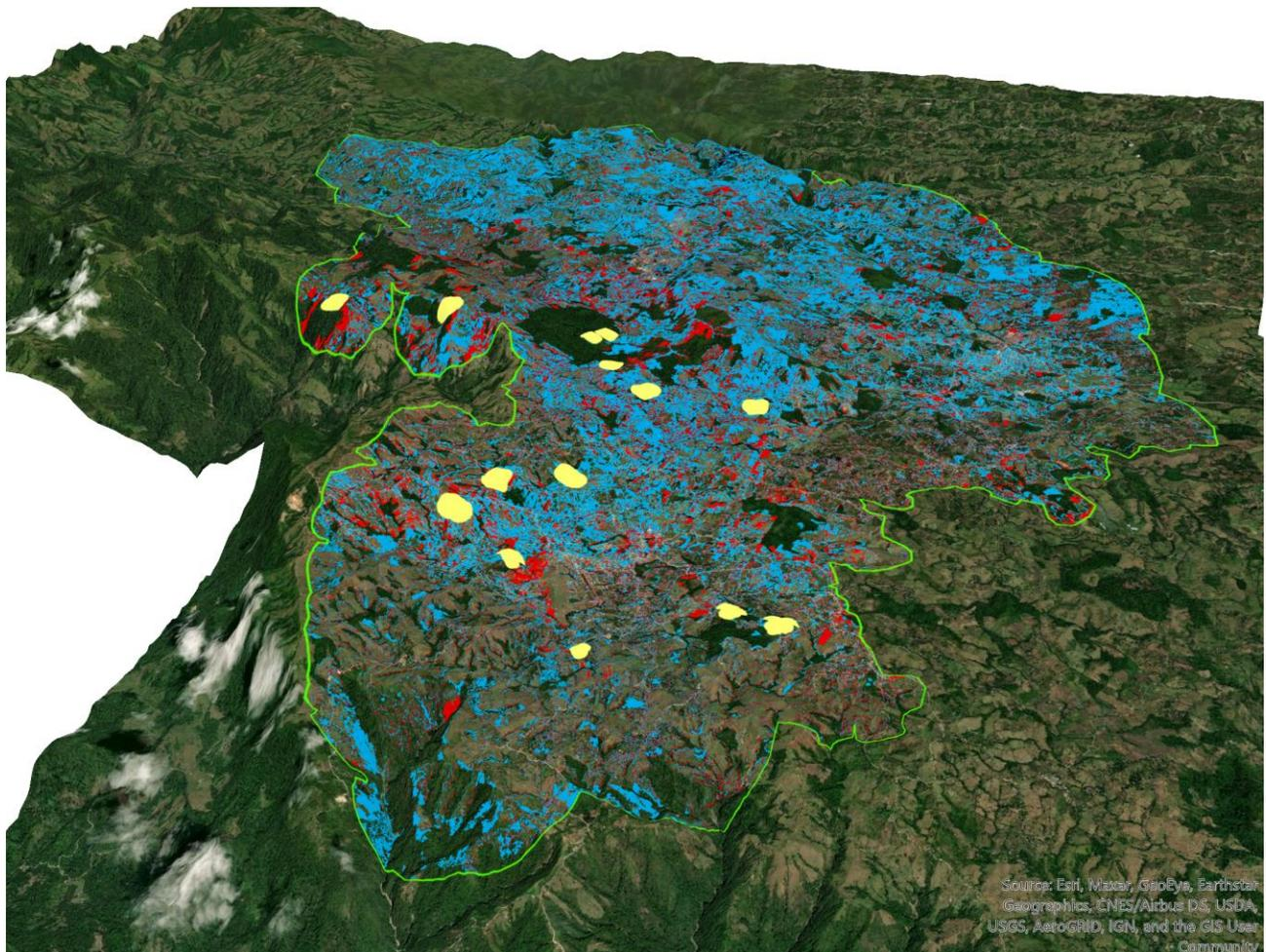
Figure 19 A 3D model of the study extent shows the treatment sites within the context of the topography. The 5-meter DEM was used to generate the surface. The surface relief was exaggerated by a factor of 2 to show the variation in landscape better. Areas in yellow are the location of the treatment sites. Blue regions are regions that experienced a gain in forest cover, and the red areas are those that suffered a loss in forest cover.
