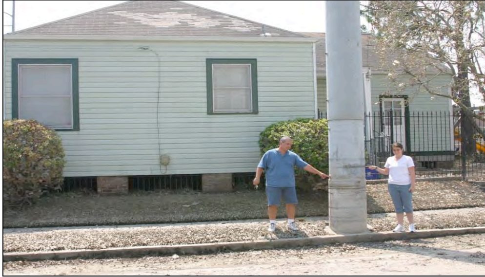
Figure 3 HWMs from Two Different Flood Events (Julie LeBlanc, USACE, New Orleans District 2005)
