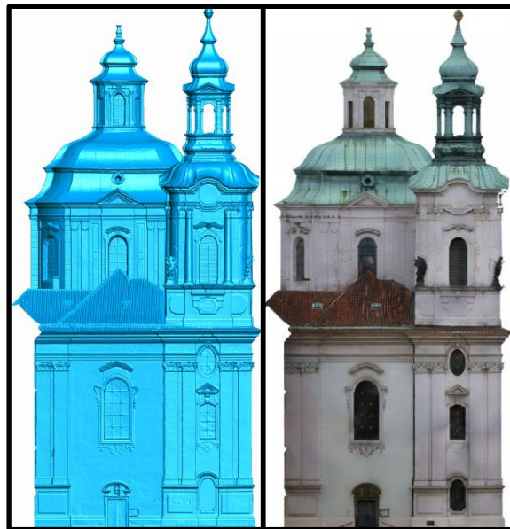
Figure 7: 3D model mesh (left) and orthoimage (right) of St. Nicholas Baroque Church.
