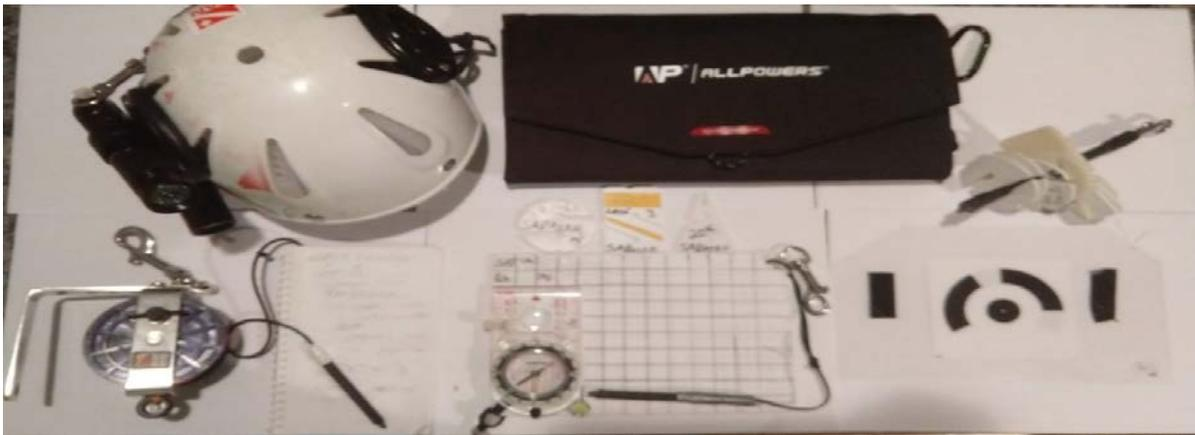
Figure 21. Photograph of traditional cave diving survey equipment including, left to right, top to bottom, light integrated helmet, 150m survey reel, solar panel, TRN H/W, survey slate with compass, level, and pencil, spare pencil and TRN markers and photogrammetry survey targets.
