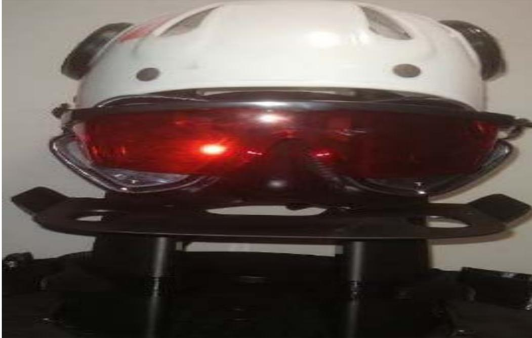
Figure 87. Laser goggles attached to cave-diving helmet for eye-safety.
