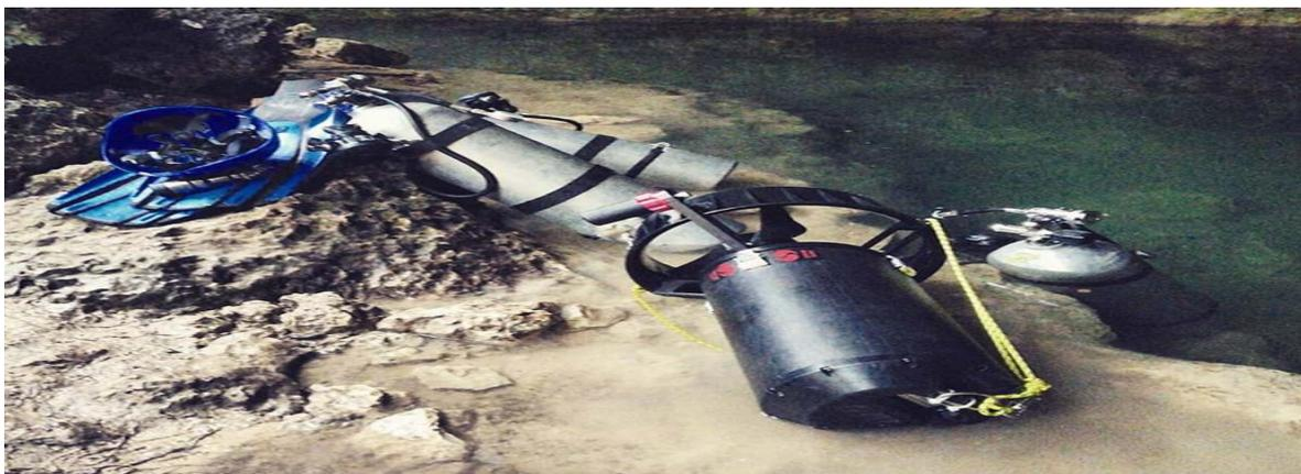
Figure 22. Photograph of diver propulsion vehicles (DPV) to reduce swimming fatigue and pen circuit self-contained breathing apparatus (SCUBA) sidemount tanks for cave survey range extension at the system entrance of Cenote Taj Mahal (Gibbs 2018).
