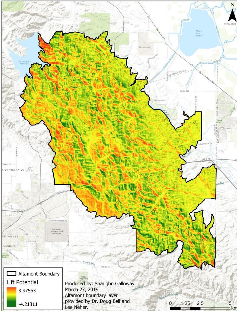
Figure 44 - Example of orographic lift from the southwest. Calculated using Equation 4.
