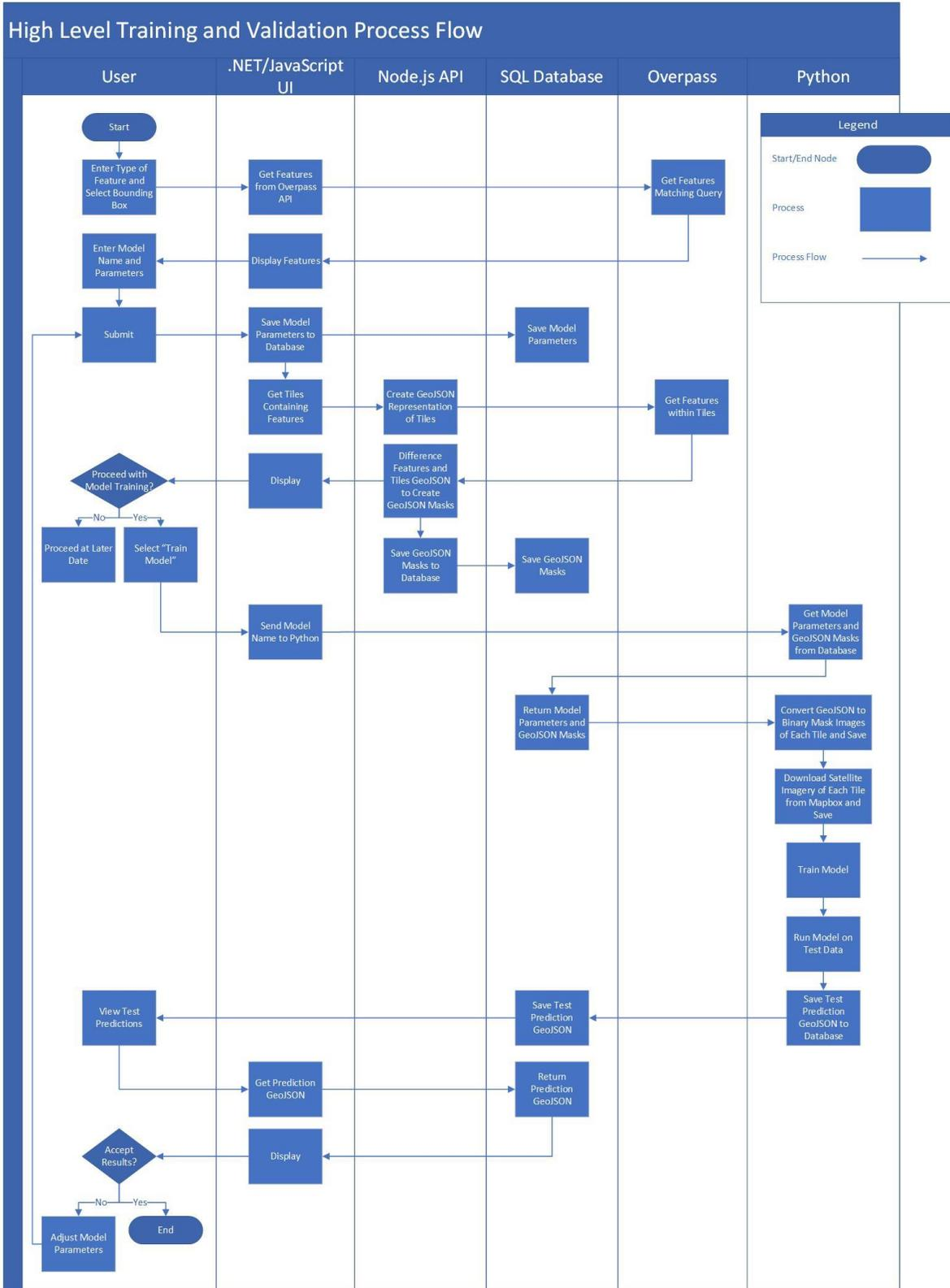
Figure 18 High Level Training and Validation Process Flow
