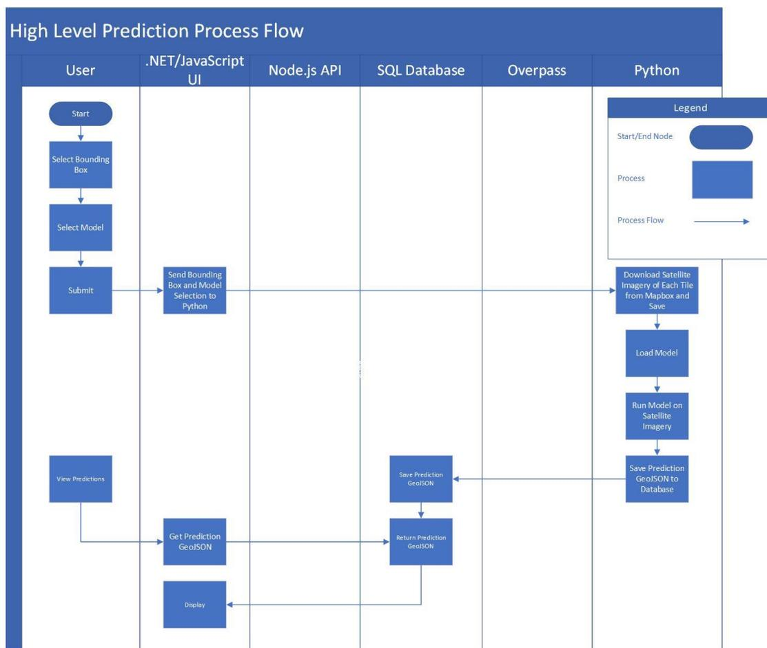
Figure 19 High Level Prediction Process Flow
