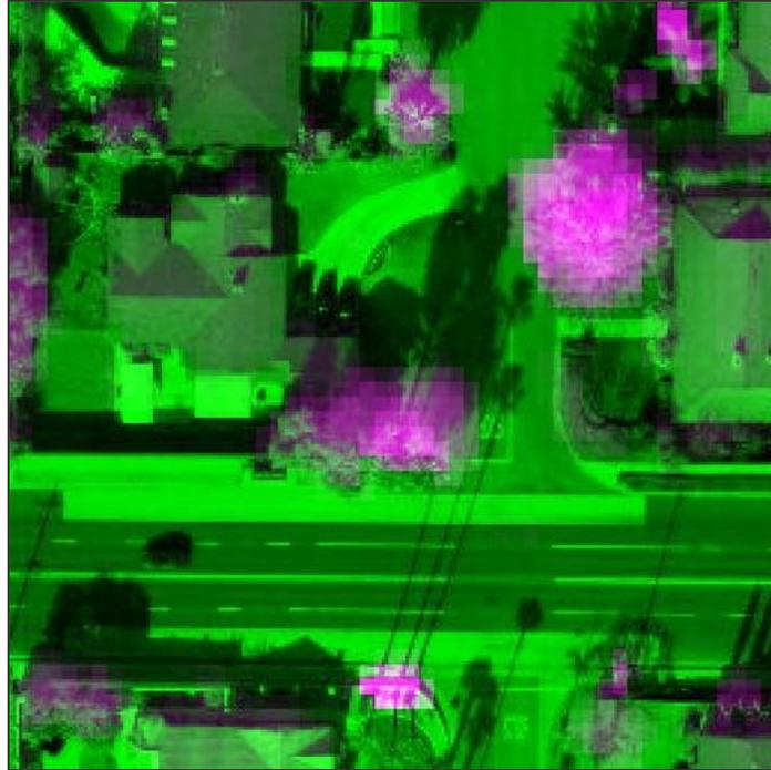
**Figure 13 LiDAR data overlaid over a 1 ft orthoimage**
