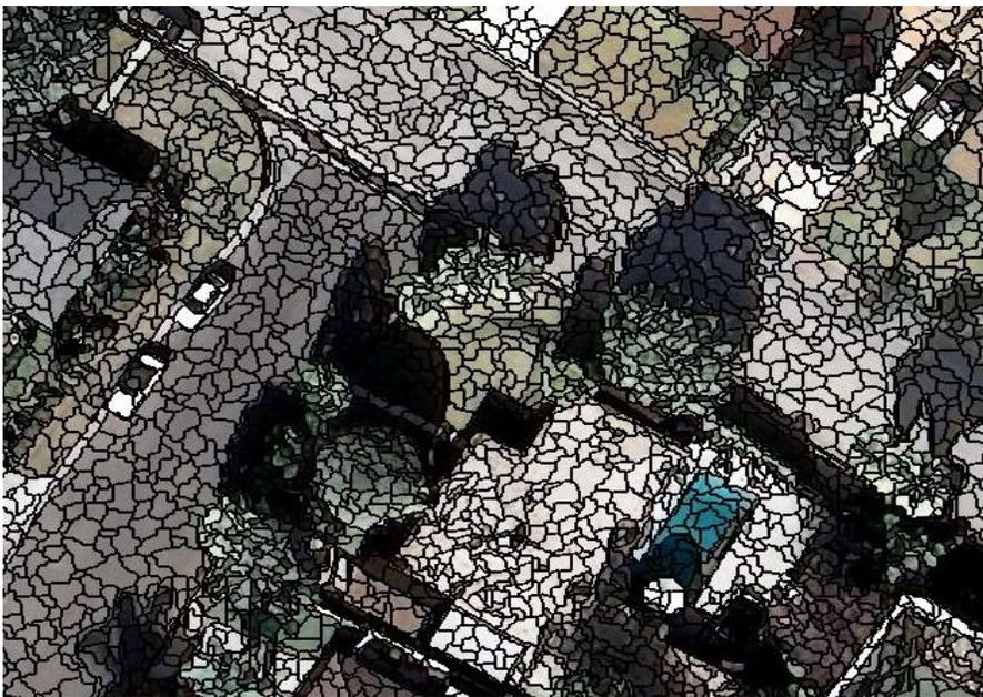
**Figure 8 Example of multi-resolution segmentation**
