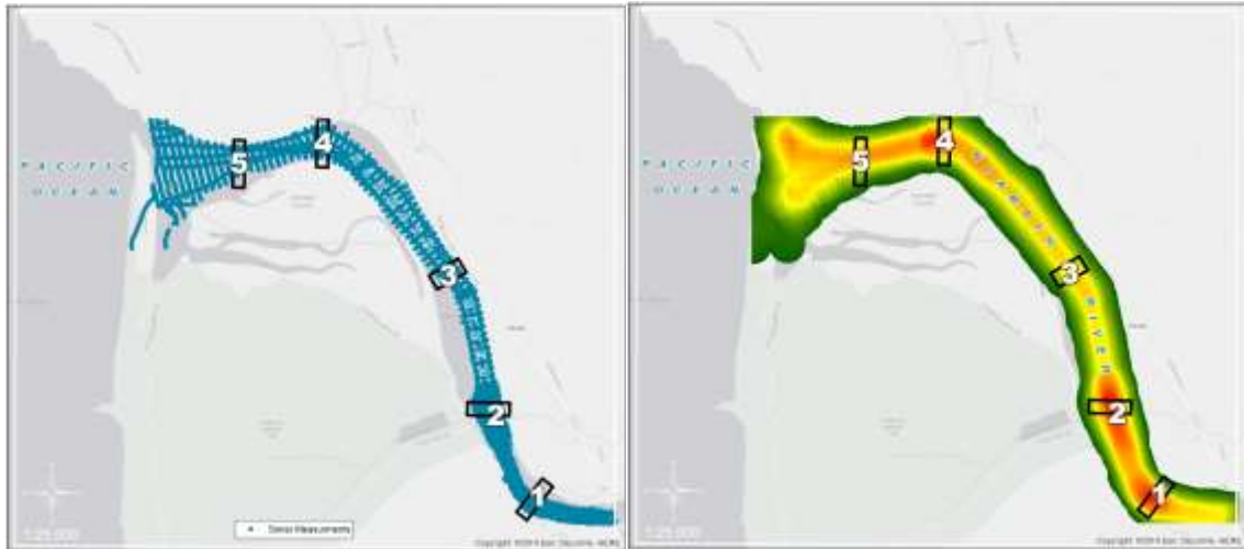
Figure 5: (Left) Individual Sonar point measurements. (Right) Density map of the Sonar measurements averaging 9.68 points per square foot
