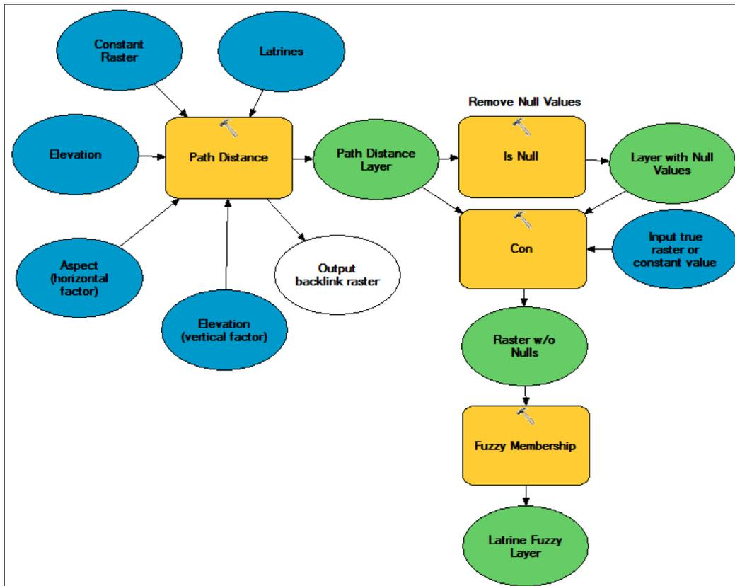
Figure 11 Overview of Contaminant Flow Analysis
