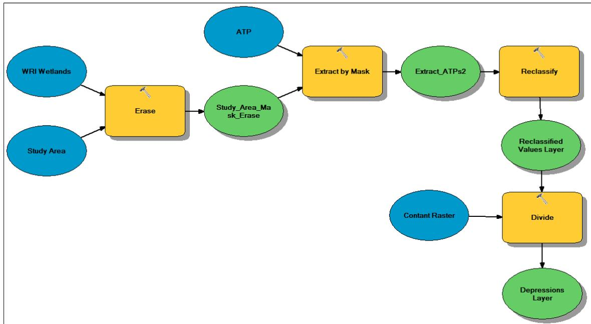
**Figure 16 Overview of Process to Create Depressions Layer**
