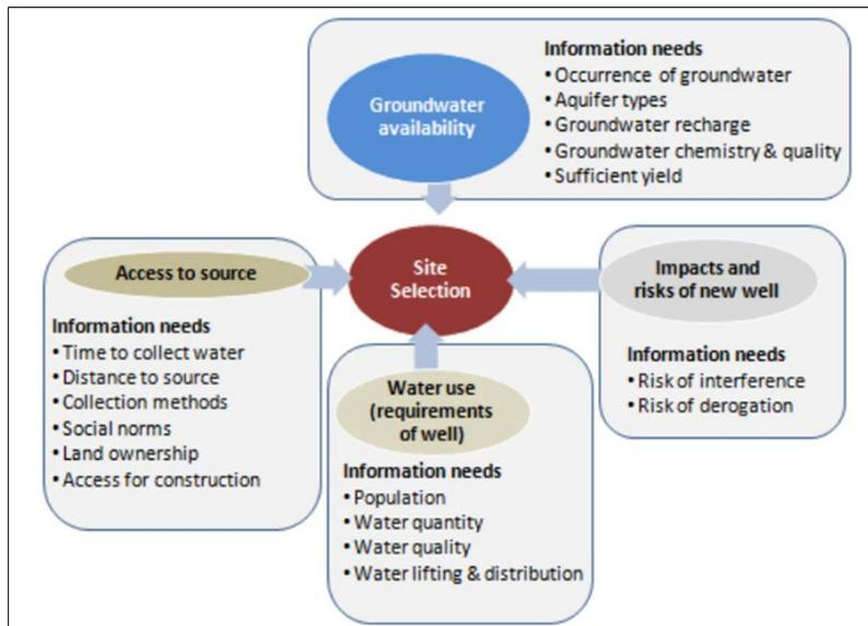
**Figure 3 Components of current well site selection**
