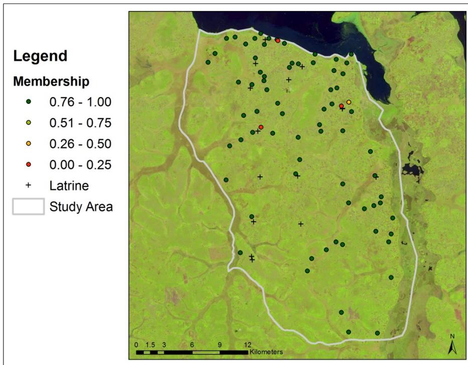
**Figure 28 Existing Wells with Contaminant Flow Membership Value**
