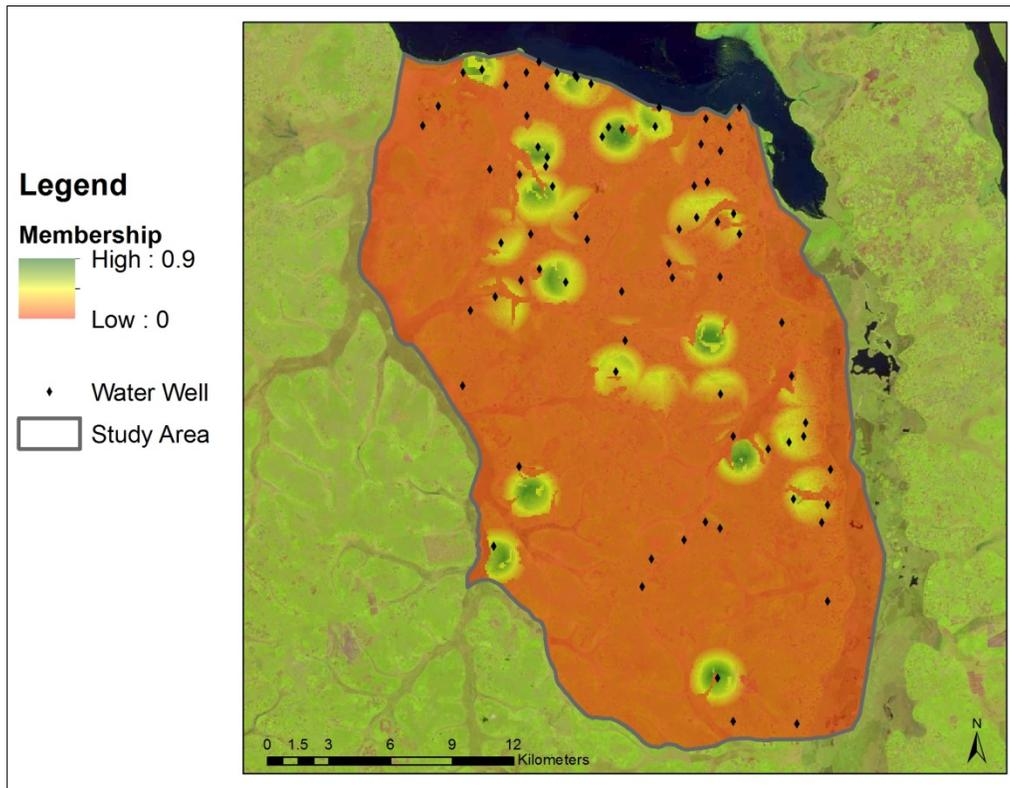
**Figure 27 Refined Suitability Map with Existing Wells**
