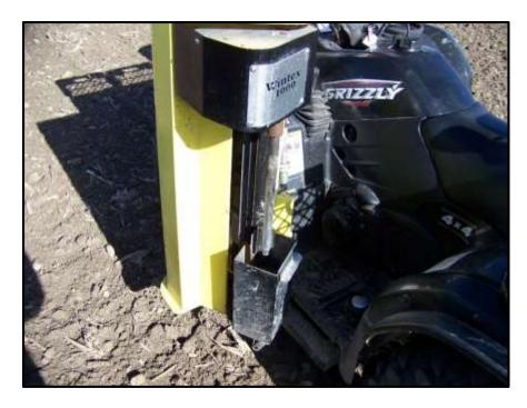
Figure 15: Automatic soil sampler mounted on ATV
