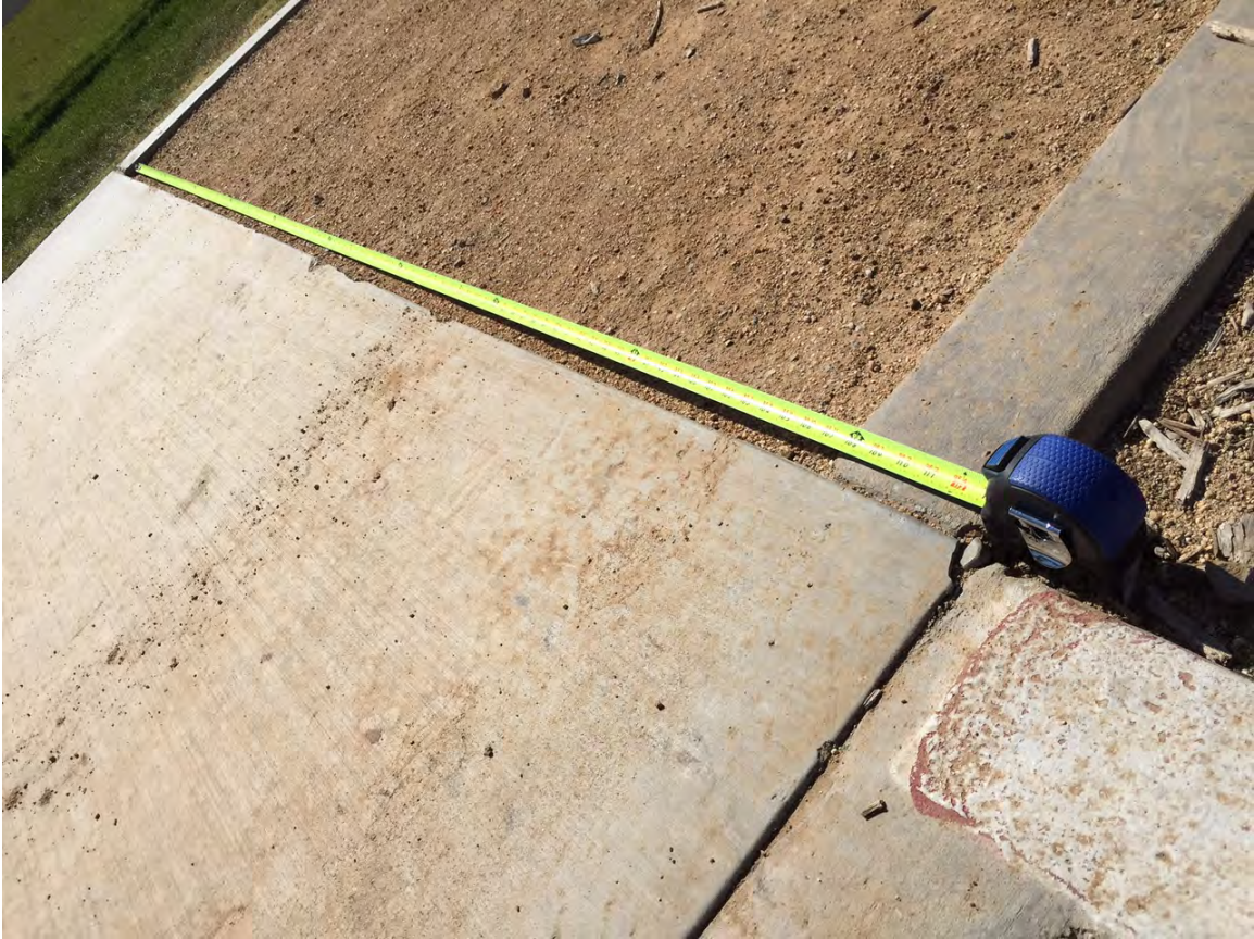
Figure 4.6 Tape measure being used to measure the width of the dirt trail to compare to ground truth data for accuracy purposes
