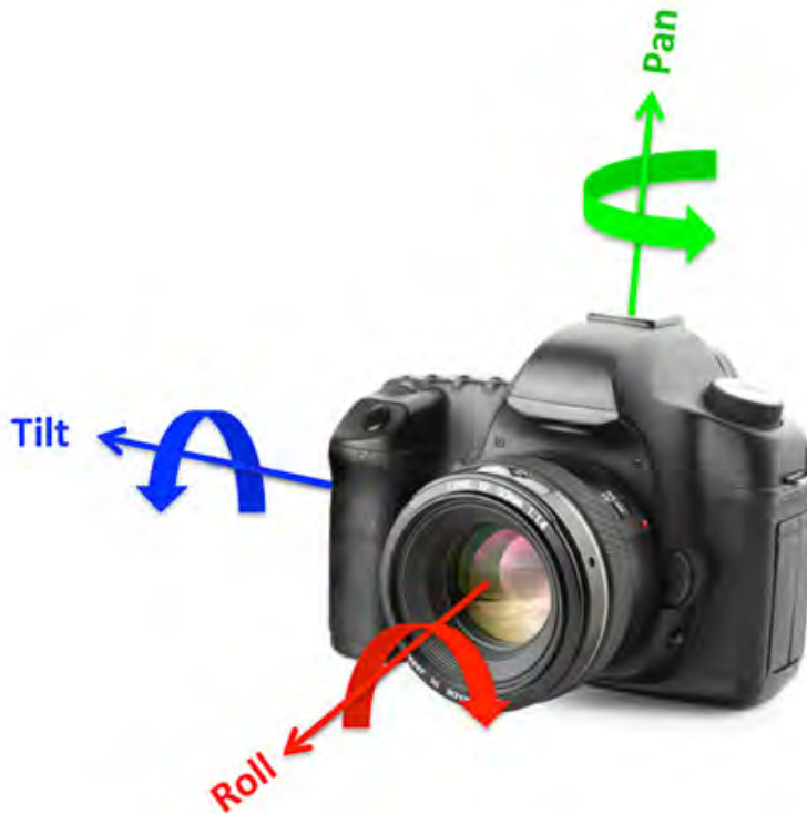
Figure 3.5 Tilt, Roll, and Pan movements in relation to a camera. (Source: https://luminous-landscape.com/landscape-aerial-photography-using-unmanned-aerial-vehicles )
