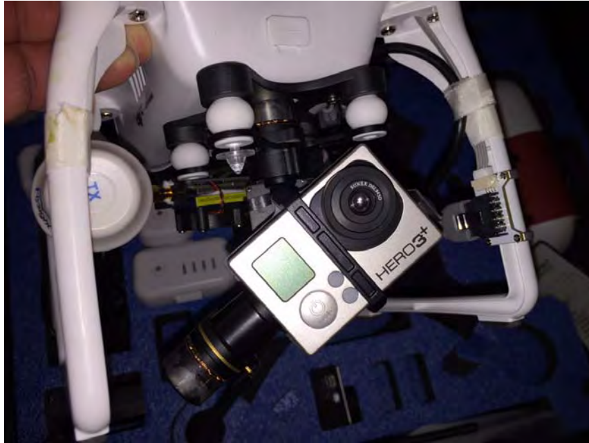
Figure 3.15 GoPro Hero 3+ Black Edition camera attached to DJI Zenmuse H3-3D Gimbal on DJI Phantom 2 prior to flight
