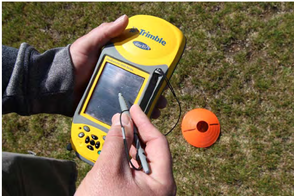
Figure 3.13 Collecting positional data for an orange soccer cone being used as a GCP at Deleo Regional Sports Park
