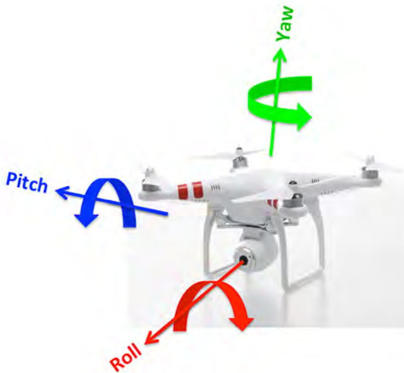
Figure 3.4 Pitch, Roll, and Yaw on a DJI Phantom Vision. (Source: https://luminous-landscape.com/landscape-aerial-photography-using-unmanned-aerial-vehicles/ )
