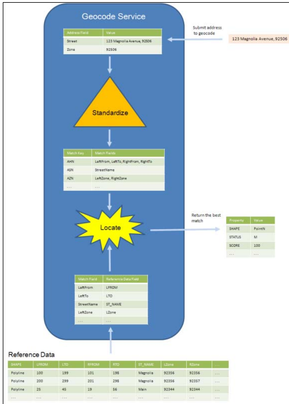
Figure 4. Diagram of a geocoding service in progress (Esri 2015)
