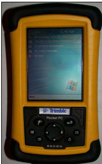
The Trimble Recon™ (left) is a sophisticated device with integrated data collection capability. An electronic version of SAGE has been developed for use on this portable GPS device.
