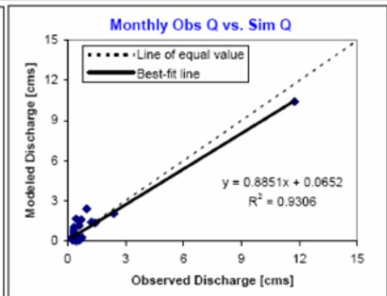
Figure A-3 Calibration results for VCWPD776 at Revolon Slough at Laguna Rd
