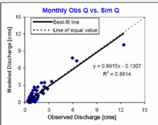
Figure A-2 Calibration results for USGS 11106400/800 at Conejo Creek above HW 101 CA
