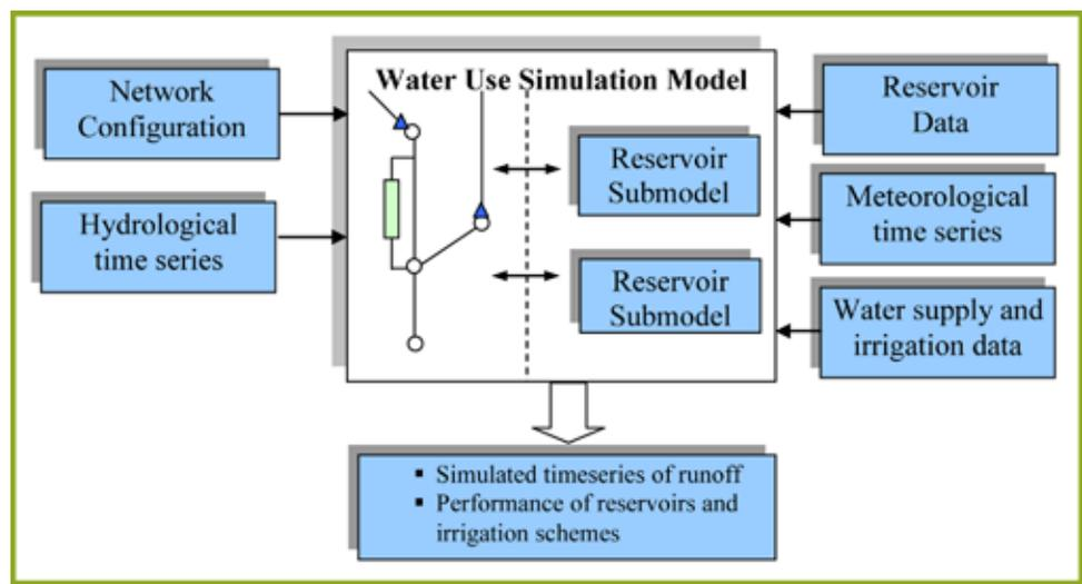
Figure 1 MIKE BASIN's water allocation modeling structure (DHI 2007)
