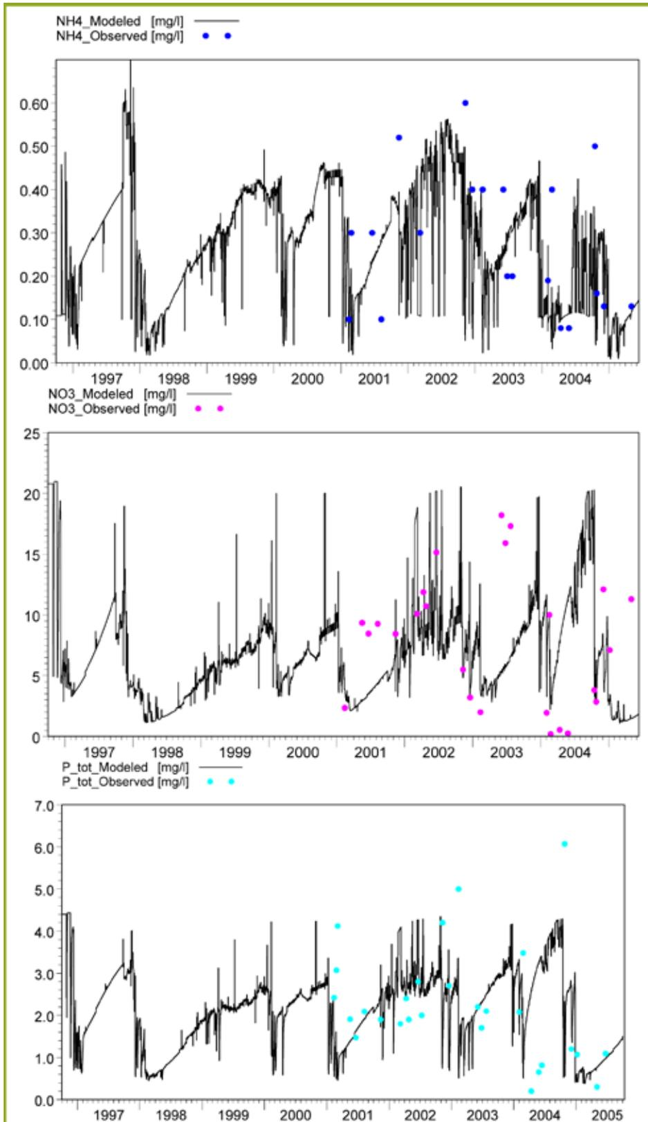
Figure B-2 Time Series comparison of modeled and observed NH4, NO3 and total P at the ME-CC mass emission site (N253)
