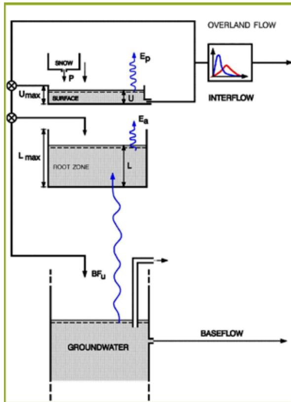
Figure 5 NAM model schematic
