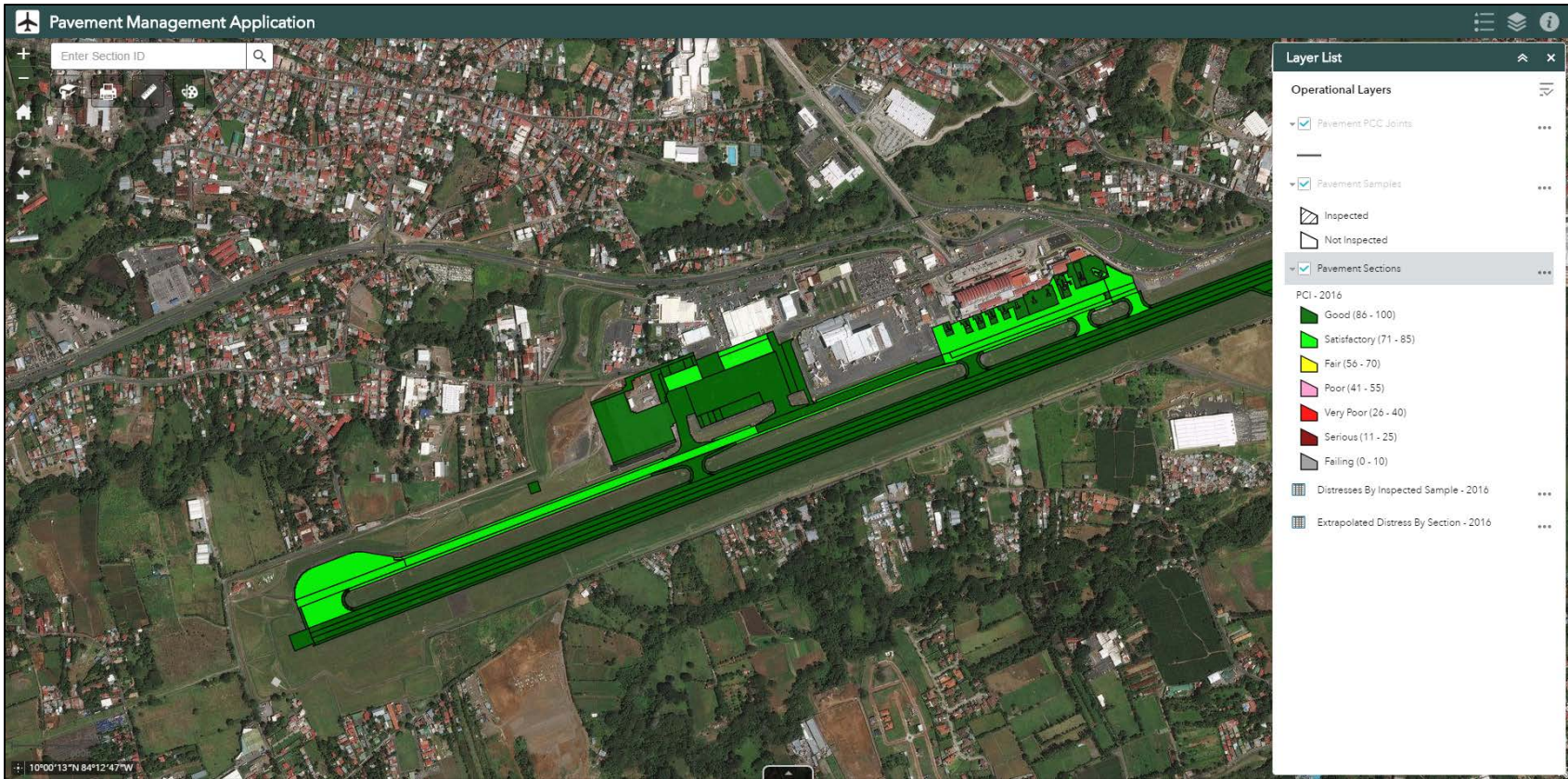
Figure 13. Airport Pavement Management Web GIS Application
