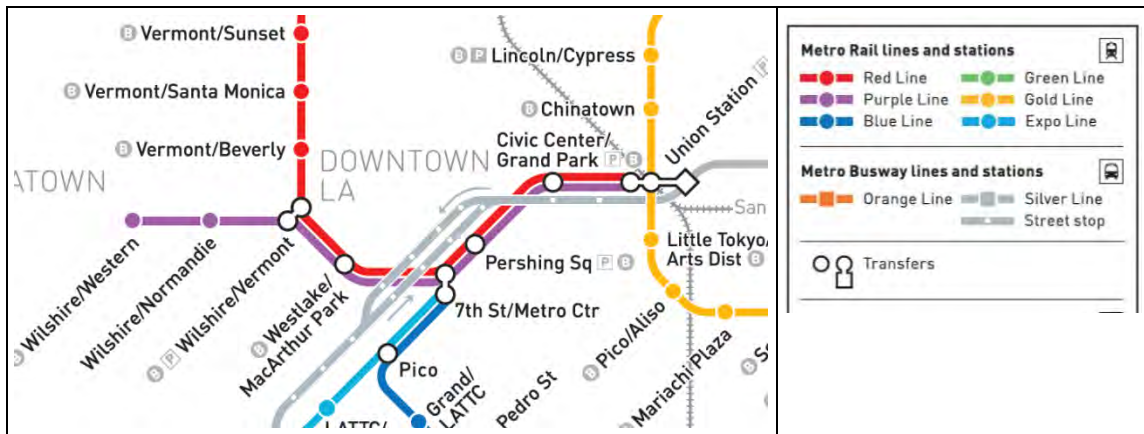
Figure 29 Single and multi-point transfer stations. Source: Metro 2015
