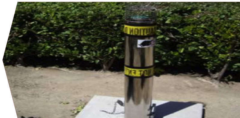
FIG. 5: Evapotranspiration Gauge that Uses Atmospheric Conditions to Calibrate the Minimum Necessary Irrigation for an Area on the University Park Campus
