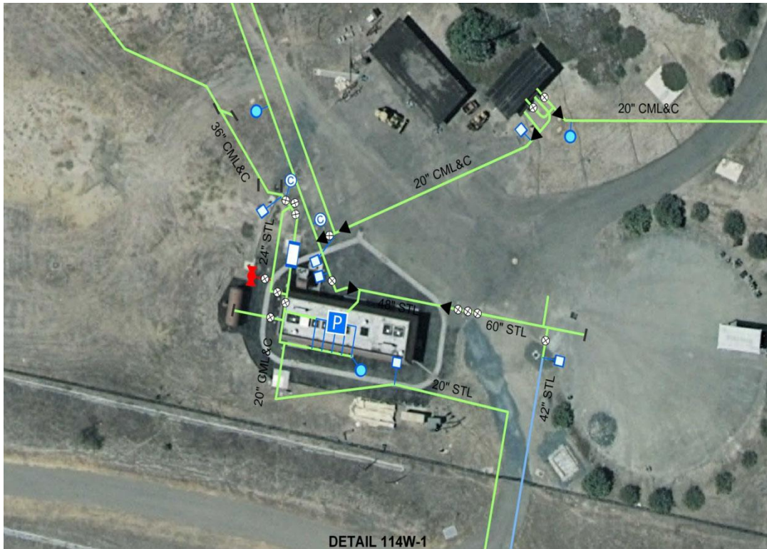
Figure 3 – Pump Station 711-1. Source: Otay Water District (2010).
