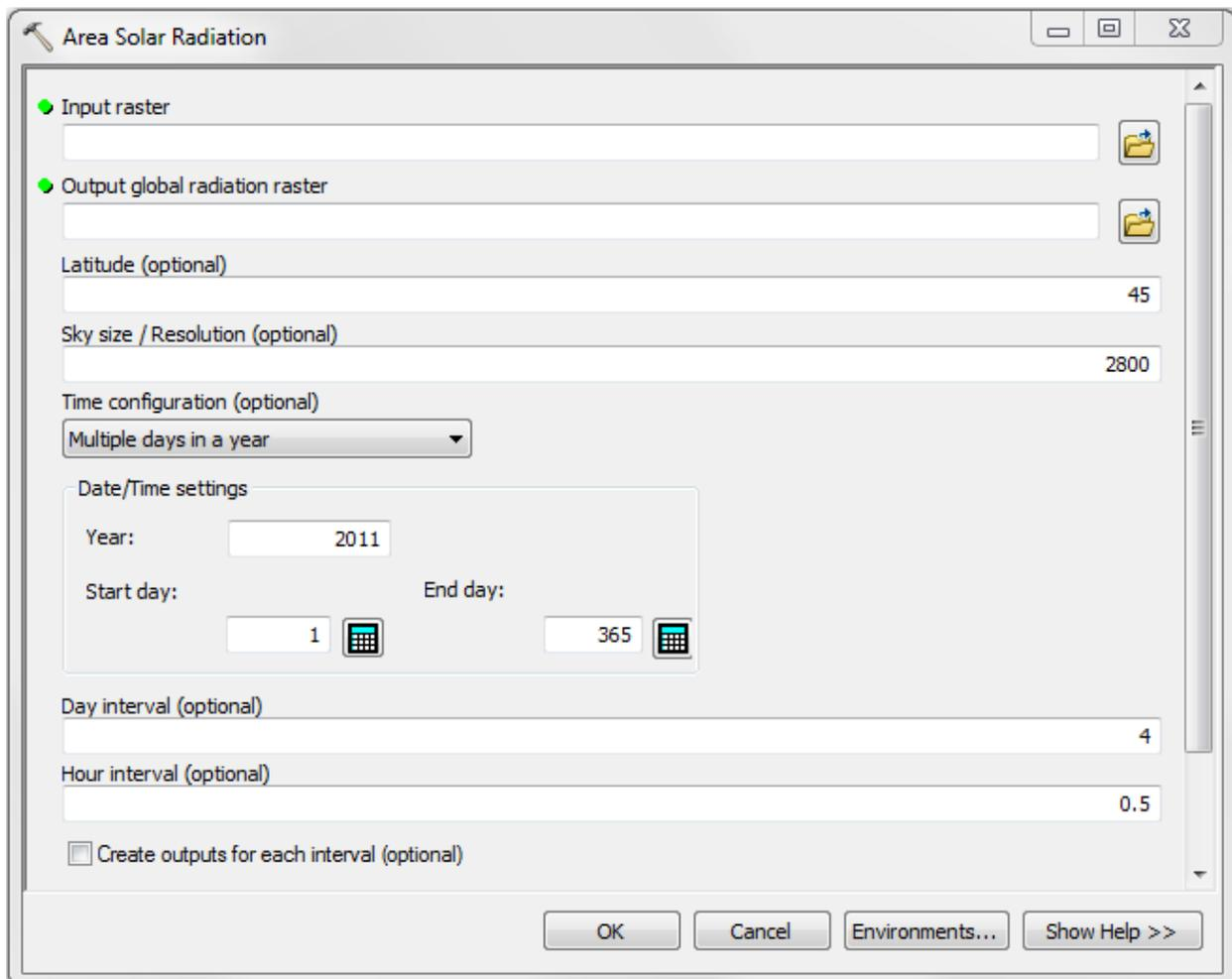
Figure 5 - Area Solar Radiation Tool Parameters
