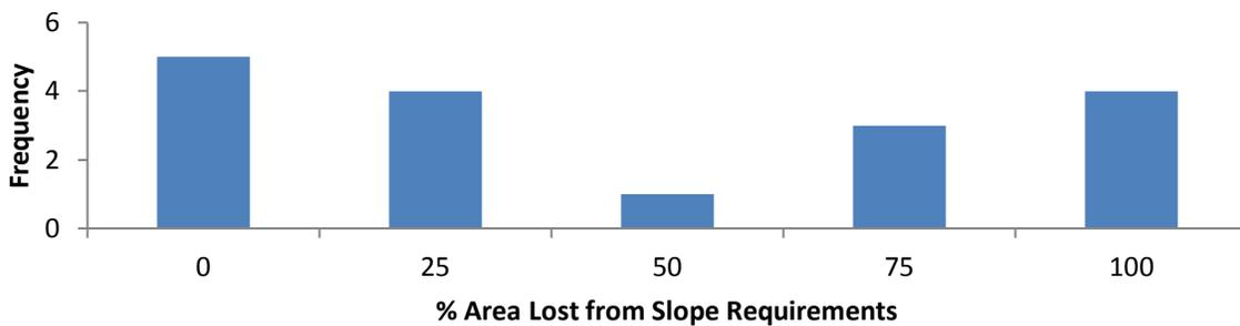
Figure 8 - Percentage of Area Remaining After Slope Analysis for Dish-Stirling Installations
