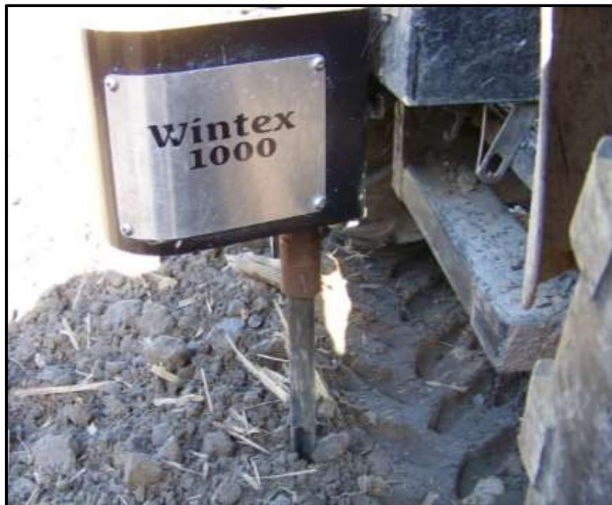
**Figure 16:** Automatic sampler obtaining a soil probe
