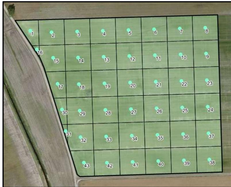
**Figure 20:** One acre systematic aligned sampling procedure used as “gold” standard
