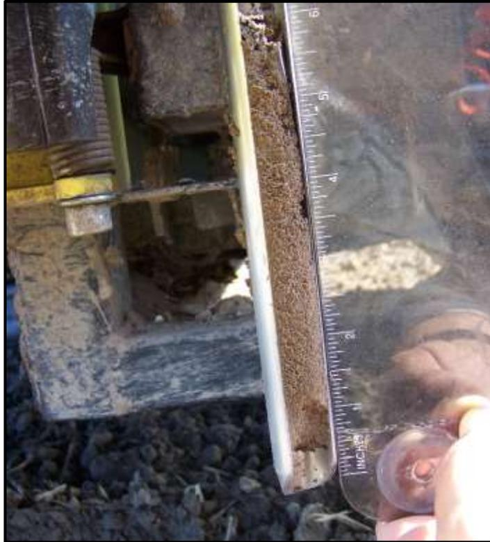
**Figure 17:** Assuring a 6" sample core: a full 6" core was normally obtained in the study samples. In the above photograph, the lower ½" of the core was lost due to the abrupt stop from using the "Emergency Stop/Kill Switch" button.
