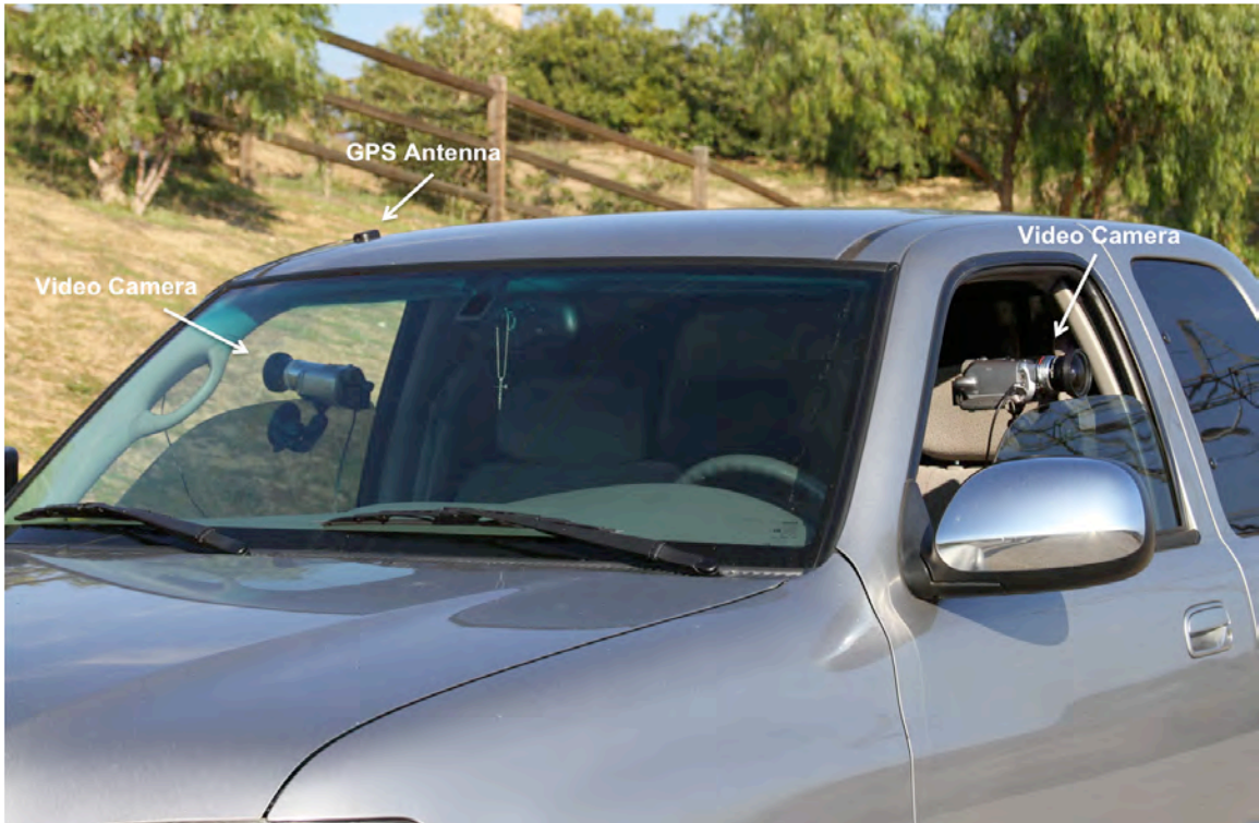
Figure 3.1: Spatial Video Acquisition System.
