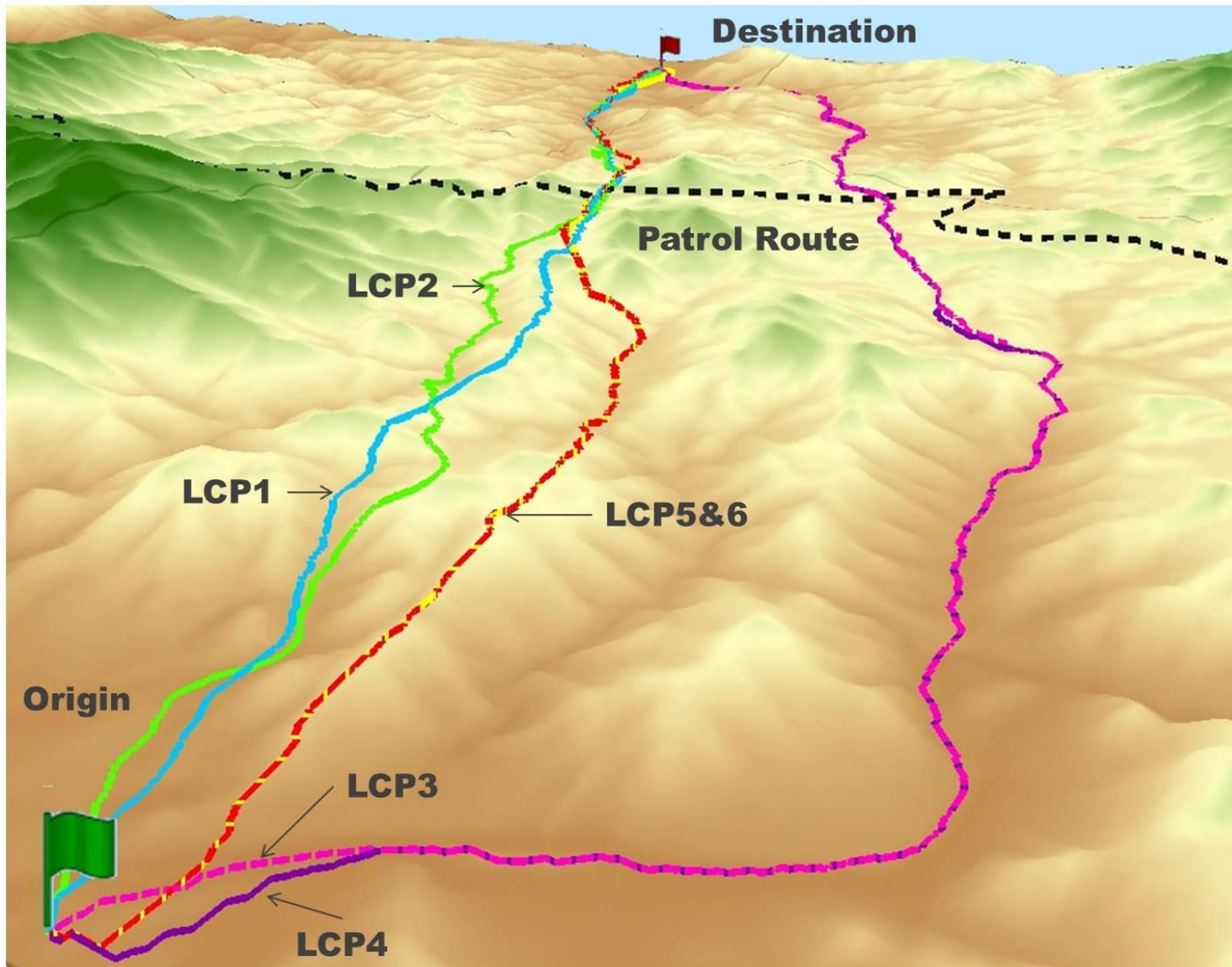
Figure 23 3D Isometric Perspective of Six Least Cost Paths. LCPs 5 and 6 Are Coincident Due to the Lack of OBP Station Proximity in this Area
