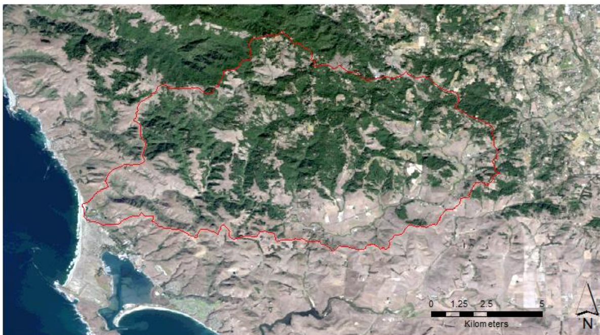
Figure 2. The Salmon Creek Watershed study area, Sonoma County, California. Image is a window, or sub-scene, of Landsat 8's OLI instrument Path 045, Row 033 from bands 2, 3, and 4, day 289. The Salmon Creek Watershed is outlined in red.
